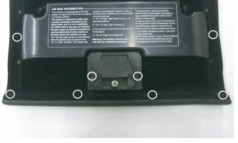
Step 3. Carefully grind or cut away remnants of factory stop arms from outside cover on both sides. It may also be necessary to trim some of the leather.
