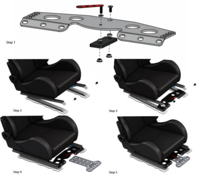
This mount may or may not work on both Drivers and Passenger seats depending on your model and options. Evaluate the clearance of the components under the seats to determine what seat you will be installing on. Some models will have wiring harnesses that may need to be moved and or secured to allow for adequate clearance.
