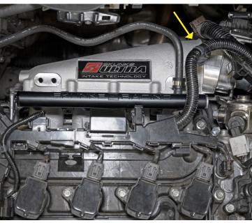
Note: Bracket Holding Harness Is Now Removed, Leave as Shown in Picture SKUNK 2 FUEL RAIL SOLD SEPARATE P/N: 350-05-1000
