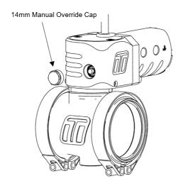
Using a ¼" drive extension with a 5mm socket, turn the manual override in a clockwise direction with your fingers until the mechanism stops rotating. In this position the butterfly valve should be home against the valve seat and will be your 0% position.
