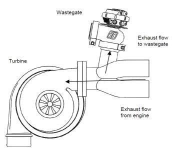
⚠ **Not Recommended** - Less than 90 Degree Mounting. An angle mounting as shown in not recommended and gives extremely
