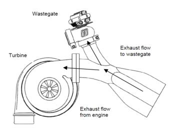
(Best Flow) Symmetric mounting allows an excellent flow of exhaust to the Waste Gate
