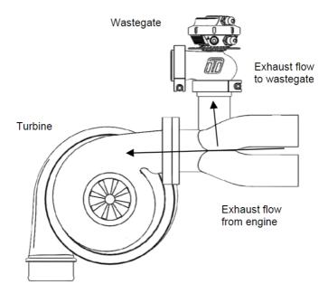
(Poor Flow) 90 Degree mounting gives poor exhaust flow to the Waste Gate and in some circumstances may contribute to over boosting.
