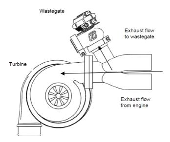
(Good Flow) Angle mounting allows a good flow of exhaust flow to the Waste Gate.
