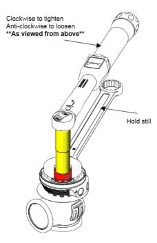
Align the valve orientation marks and confirm the diaphragm bead is seated in the groove of the actuator. Install desired spring combination. Configure Wastegate with preferred spring combination of inner, middle and outer springs
