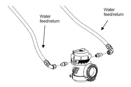
⚠ CAUTION! Confirm water is only used on the water ports of the wastegate, damage to your engine may result in failure to correctly connect water cooling.
