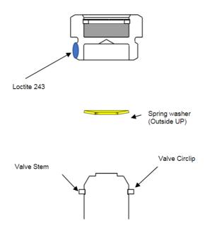
Sit the new spring washer into the valve retaining cap with the centre of the washer pointing out of the cap. Apply a dab of blue 243 Loctite to the lower threads of the valve retaining cap and screw into the diaphragm. Support the diaphragm with the supplied tool and tighten the valve retaining cap to 20N.m (15ft/lbs)
