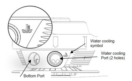
Fit water cooling port fittings Prior to mounting the wastegate, install 1/8" NPT fittings into the water ports, apply thread lubricant and screw in clockwise until finger tight, then tighten further 1-2 turns for seal. Choose feed and drain source for the water and connect to the wastegate. Turbosmart recommends -4 SAE fittings and hose compatible with coolant.
