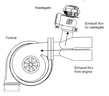
▲ Not Recommended - Less than 90 Degree Mounting. An angle mounting as shown in not recommended and gives extremely poor exhaust flow to the Straight Gate which can contribute to poor boost control and over boosting.
