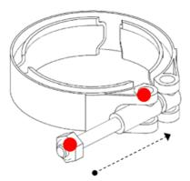
△ CAUTION! Do not forget to put the valve seat into the body before mounting the unit on the exhaust manifold. Using the 3/8" deep socket and a torque wrench tighten the V-Band to 7N.m (5 ft/lbs).
