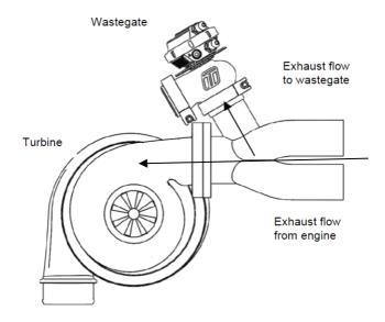
(Good Flow) Angle mounting allows a good flow of exhaust flow to the Straight Gate.
