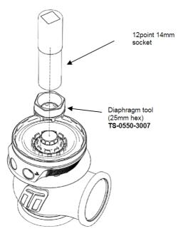
Clear any Loctite and debris from the thread in the diaphragm support, Note careful not to get chemicals onto the diaphragm as this may damage the diaphragm.
