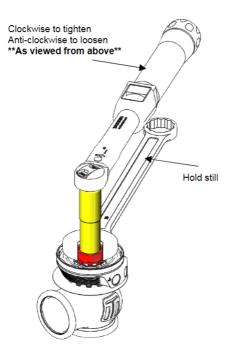
Align the valve orientation marks and confirm the diaphragm bead is seated in the groove of the actuator. Install desired spring combination. Configure Wastegate with preferred spring combination of inner, middle and outer springs
