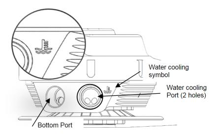
Fit water cooling port fittings Prior to mounting the wastegate, install 1/8" NPT fittings into the water ports, apply thread lubricant and screw in clockwise until finger tight, then tighten further 1-2 turns for seal. Choose feed and drain source for the water and connect to the wastegate. Turbosmart recommends -4 SAE fittings and hose compatible with coolant.
