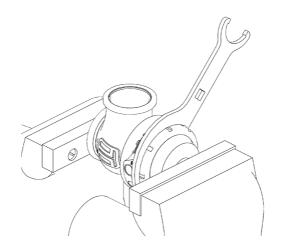
Reinstall fittings to the cap of the wastegate using fresh Loctite 567 thread sealant.
