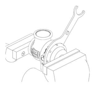
Reinstall fittings to the cap of the wastegate using fresh sealant.
