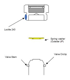
Sit the new spring washer into the valve retaining cap with the centre of the washer pointing out of the cap. Apply a dab of blue 243 Loctite to the lower threads of the valve retaining cap and screw into the diaphragm. Support the diaphragm with the supplied tool and tighten the valve retaining cap to 20N.m (15ft/lbs)
