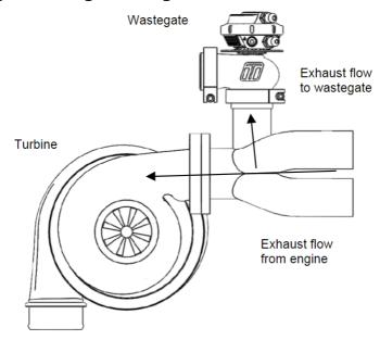
(Poor Flow) 90 Degree mounting gives poor exhaust flow to the Straight Gate and in some circumstances may contribute to over boosting.
