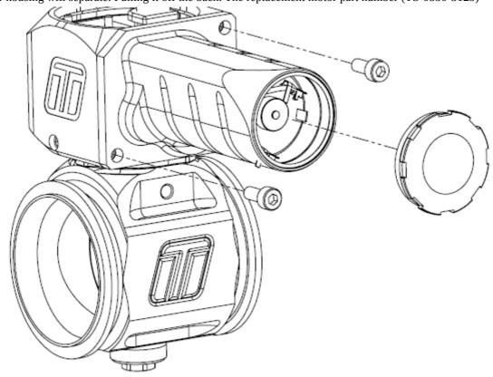
A 2.5mm Allen key will be required to remove the motor screws. With both undone. The motor can be lightly pushed out. When reinstalling, use a small application of Loctite 243
