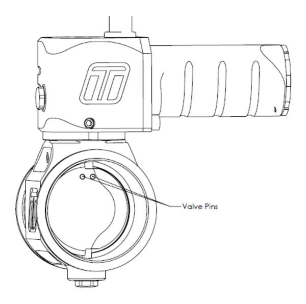
Using a 4mm allen key and a torque wrench tighten the V-Band to 3N.m (2 ft/lbs). Ensure the boostgate is seated in the v-band flange correctly while torquing the screw to prevent intake leaks.
