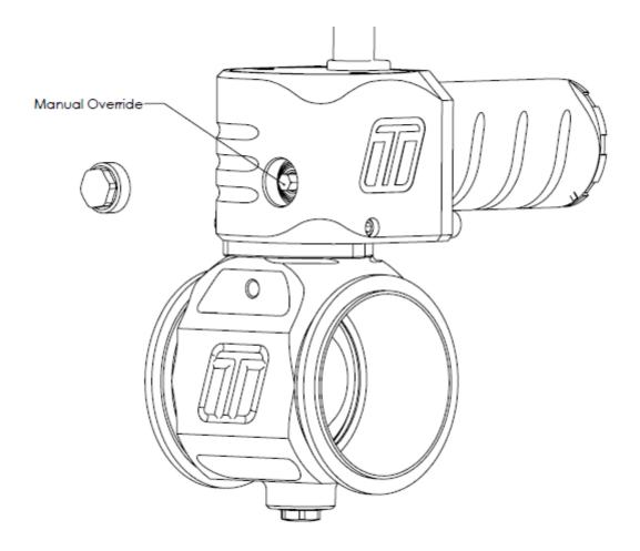
Using a ¼" drive extension with a 5mm socket, turn the manual override in a clockwise direction with your fingers until the mechanism stops rotating. In this position the butterfly valve should be seated against the valve seat and will be your 0% position.
