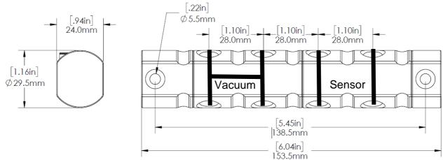
Each Sensor Input has 1 input and 1 Sensor output totalling 2 Possible Inputs. Vacuum is shared between 4 Ports.
