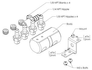
Vacuum Source is Common Shared between 1/4NPT Input and 4 x 1/8 NPT Output
