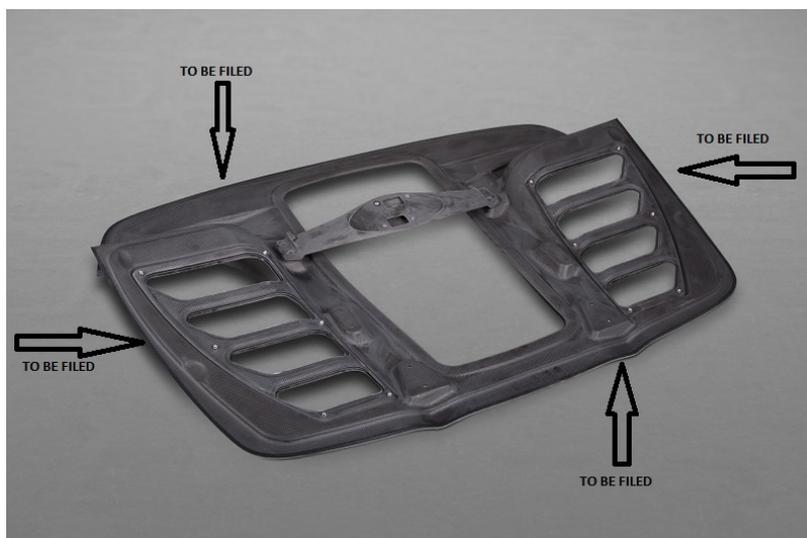
Install the hood on the car and file all the edges to make sure all the lines are the same size, make sure the hood's lines are following the lines on the car
