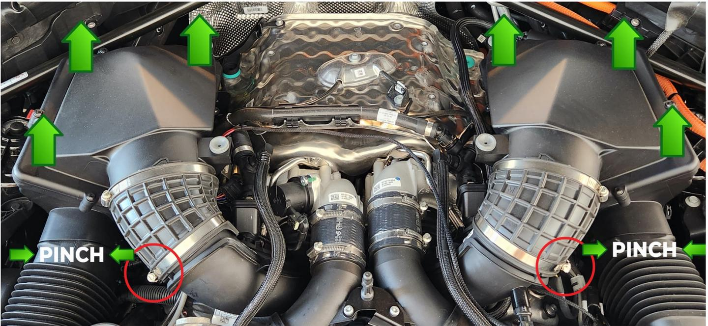
Now remove the right side (facing the engine) turbo inlet but unplugging the circled temperature sensor, then the PCV hose by pulling up on the circlip. Next pull up on the large circlip on the turbo inlet and pull it towards the front of the vehicle to remove.
