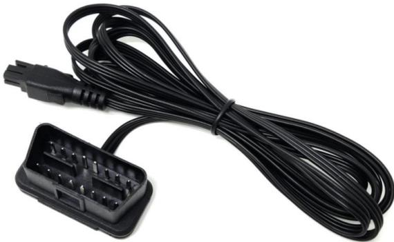
The easiest way to route to the engine bay is around the door jamb. Alternatively, it can be run through the firewall into the pedal area if there are any unused grommets. Finally plug OBDII into JB4 harness, note correct clip over notch orientation. If no data appears in JB4 app once connected an issue with the OBDII connection is usually the culprit.
