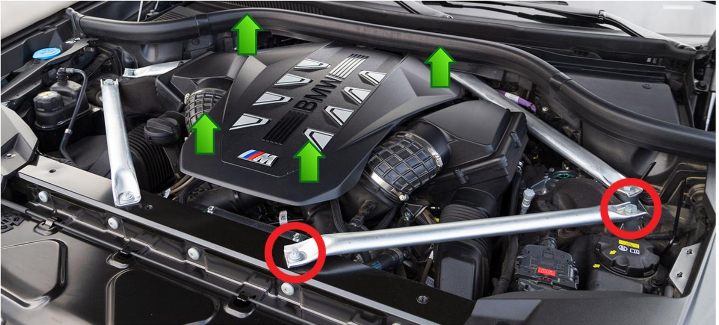
2023+ BMW XM remove the engine cover by pulling up on the front and then pulling up on the back. Next remove the front strut brace.
