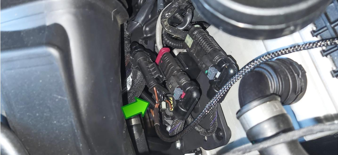
Now unplug the factory MAP connector on the right side of the right intercooler. It's the 3<sup>rd</sup> plug down.
