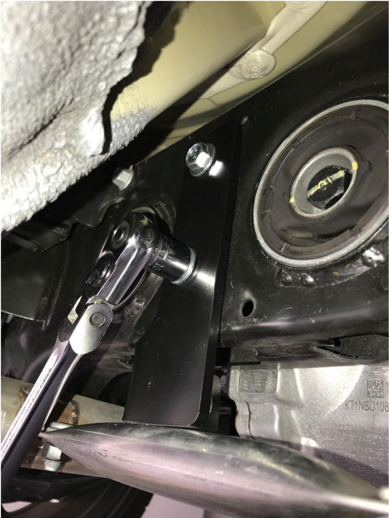
Attach the large bottom brace to the L shaped bracket using the last two provided bolts and lock nuts.
