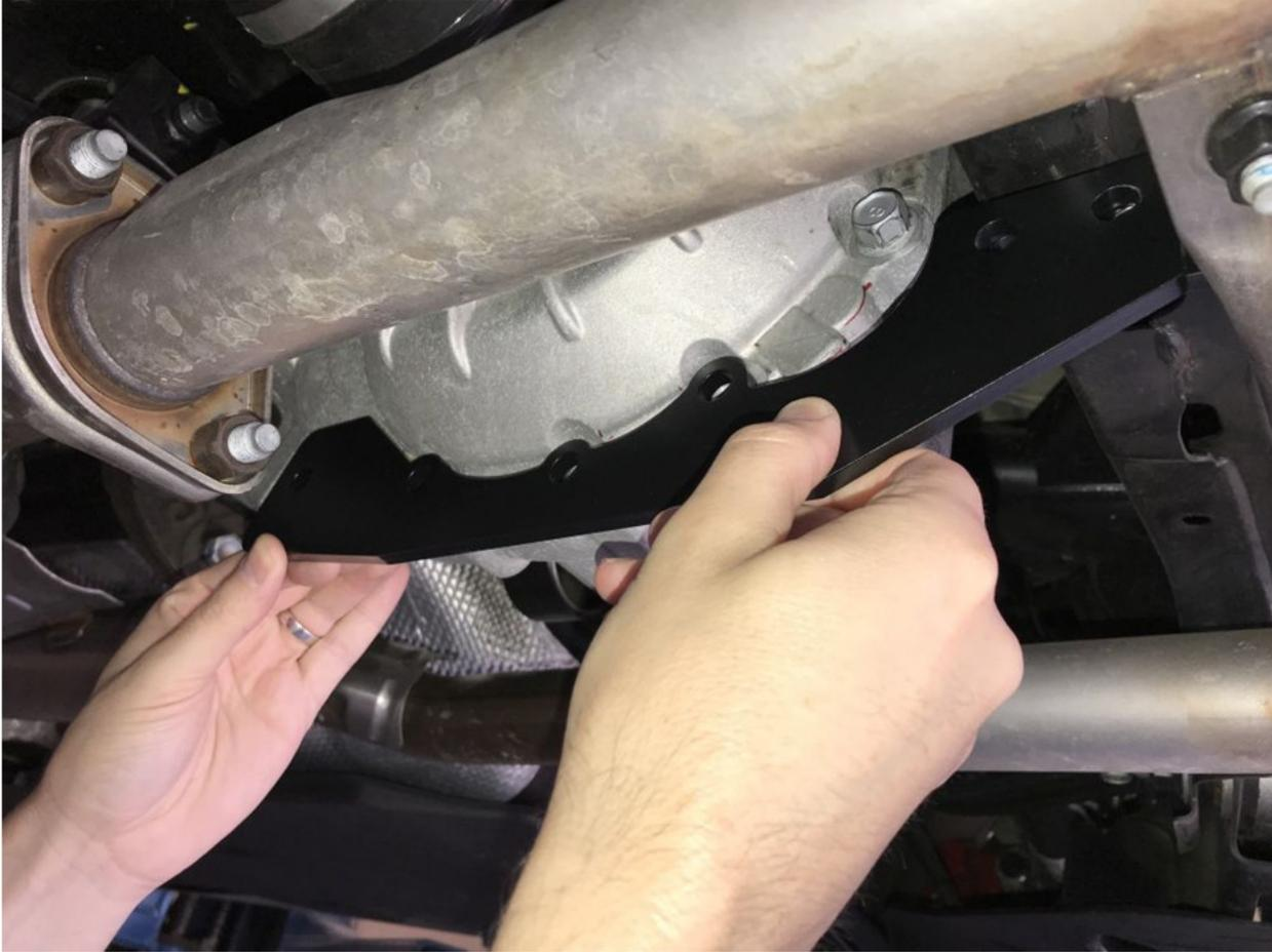
Slide the smaller bracket with the two welded nuts into the rear subframe slot as shown. The L shaped bracket will be tightened down to this using the two of the four bolts provided.
