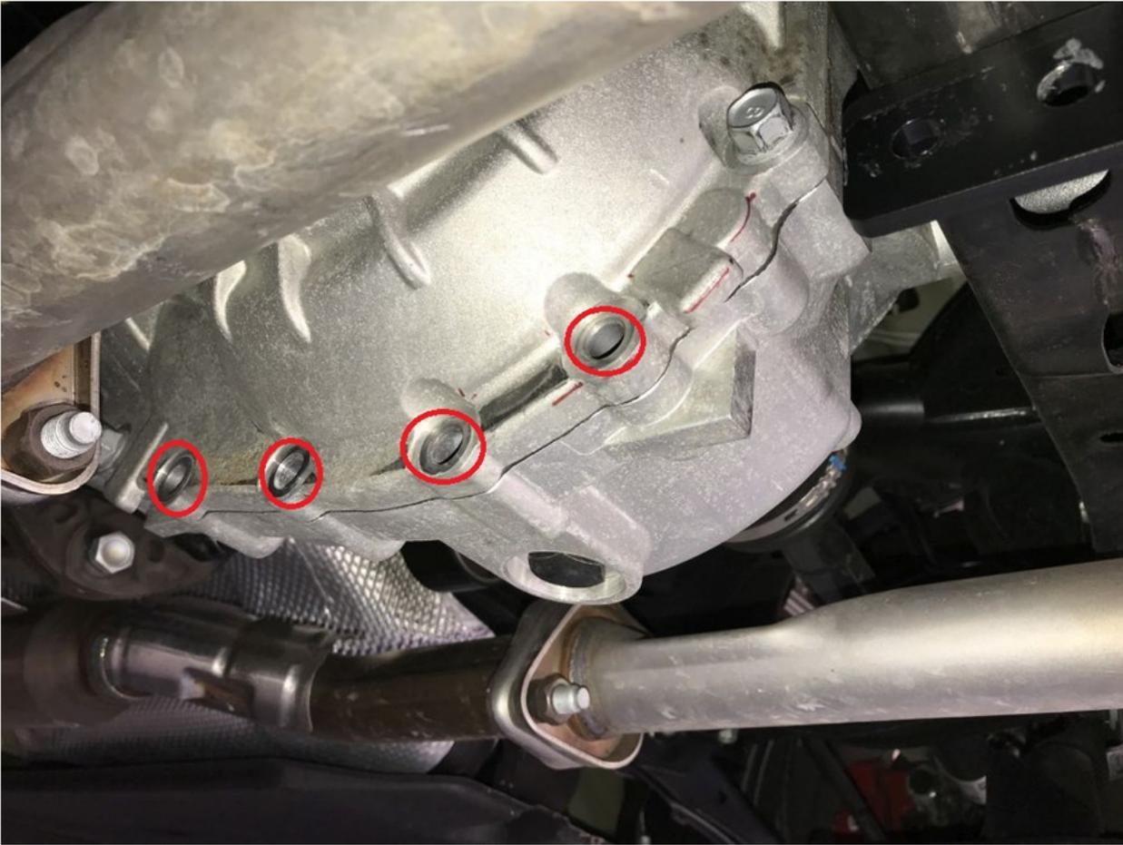
After removing the bolts, install the differential brace first onto the differential. Don't tighten anything down just yet until all diff brace pieces are on.
