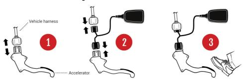
Never install or remove the PedalBox\* system with the key inserted in the ignition or the ignition system active. Always switch off the ignition and wait 5 minutes for all electrical systems to power down and fully discharge.
