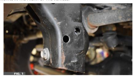
STEP 2: SLIDE SKID PLATE INTO PLACE ALIGNING THE 4 SKID PLATE MOUNTING BRACKETS HOLES WITH HOLES IN THE FRAME HORN.
