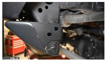
STEP 3: WITH THE SKID IN POSITION AND HOLES ALIGNED, INSTALL 1X 5/8" BOLT AND WASHER ON EITHER SIDE.
