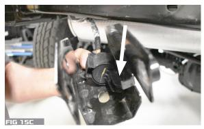
7. ROUTE WIRE HARNESS THROUGH NEW BUMPER NOTING CORRECT ORIENTATION. FIG. 16,17,18,19,20
