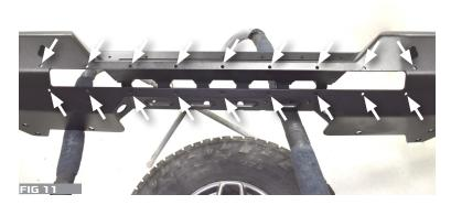
3. INSTALL THE SHORT BUMPER TRIM PLATE TO THE FRONT OF THE BUMPER USING THE PROVIDED 13 BOLTS AND NUTS. DO NOT TIGHTEN UNTIL ALL HARDWARE IS INSTALLED. FIG. 12
