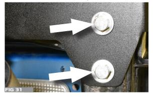
14. TO INSTALL THE 4 TOP BOLTS AND NUTS ON DRIVER AND PASSENGER SIDE OF THE BUMPER, FIRST OPEN THE REAR GATE TO ALLOW ROOM TO ACCESS THE TOP OF THE BUMPER. DO NOT TIGHTEN FIG. 32
