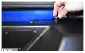
15. INSTALL 2 BOLTS AND NUTS ON BOTH SIDES OF THE BUMPER. DO NOT TIGHTEN FIG. 33
