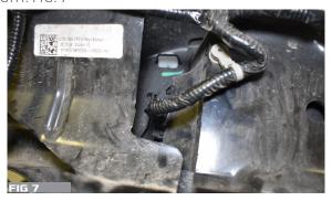
7. REMOVE THE 14 WIRE HARNESS RETAINING CLIPS TO ALLOW FOR WIRE HARNESS REMOVAL. FIG. 8,9
