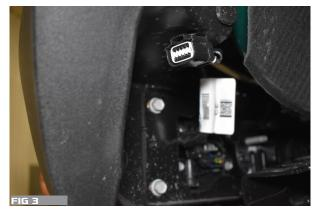
3. REMOVE 4 FRONT SKID PLATE BOLTS. LOOSEN 2 REAR SKID PLATE BOLTS, DO NOT REMOVE. FIG. 4, 5, 6
