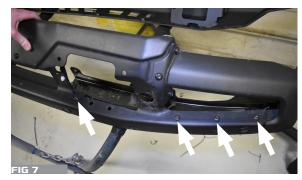
8. USE TRIM TOOL TO REMOVE ALL RETAINER CLIPS. FIG. 8 RETAINING WIRE HARNESS FIG. 9
