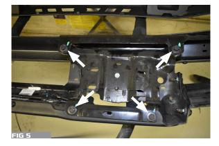
7. REMOVE THE 3 BOLTS ON TOP AND 4 BOLTS ON THE BOTTOM, REMOVE BRACKET AND SET ASIDE. FIG. 6,7
