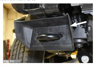
NOTE: IF NOT INSTALLING THE CRAWLTEK SKID PLATE YOU HAVE THE OPTION TO LEAVE THE OE TOW HOOKS OR REMOVE AND REPLACE THEM WITH THE PROVIDED INTERCOOLER BRACKETS. TO REPLACE THE OE TOW HOOKS WITH THE INTERCOOLER BRACKETS IT IS RECOMMENDED THAT YOU DO ONE SIDE AT A TIME TO PREVENT THE INTERCOOLER FROM FALLING OUT OF THE VEHICLE WHICH COULD RESULT IN INTERCOOLER DAMAGE.
