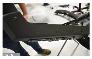
4. INSTALL THE 2 OUTER VENT GRILLS WITH THE 6 PROVIDED BOLTS. FIG. 16, 17
