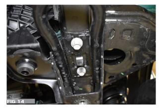
12. REMOVE INTERCOOLER RUBBER ISOLATORS ON BOTH SIDES. INSTALL SPACER ABOVE RUBBER ISOLATOR (FIG. 15A) BETWEEN INTERCOOLER AND ISOLATOR. (FIG. 15B)
