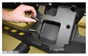
2. INSTALL CENTER VENT GRILL USING THE 6 PROVIDED BOLTS AND NUTS. SNUG BUT DO NOT TIGHTEN UNTIL ALL BOLTS ARE INSTALLED. FIG. 14
