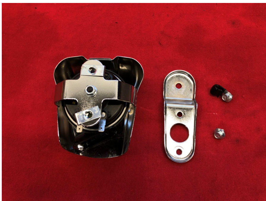
Step 8: Remove horn bracket from horn as shown.
