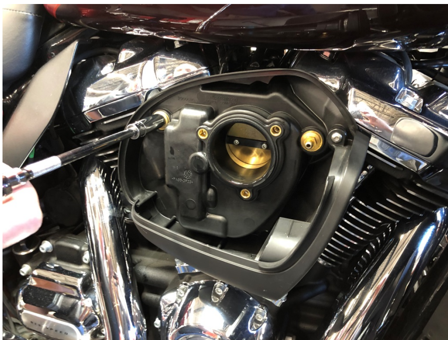
Step 3: Remove air pan.
