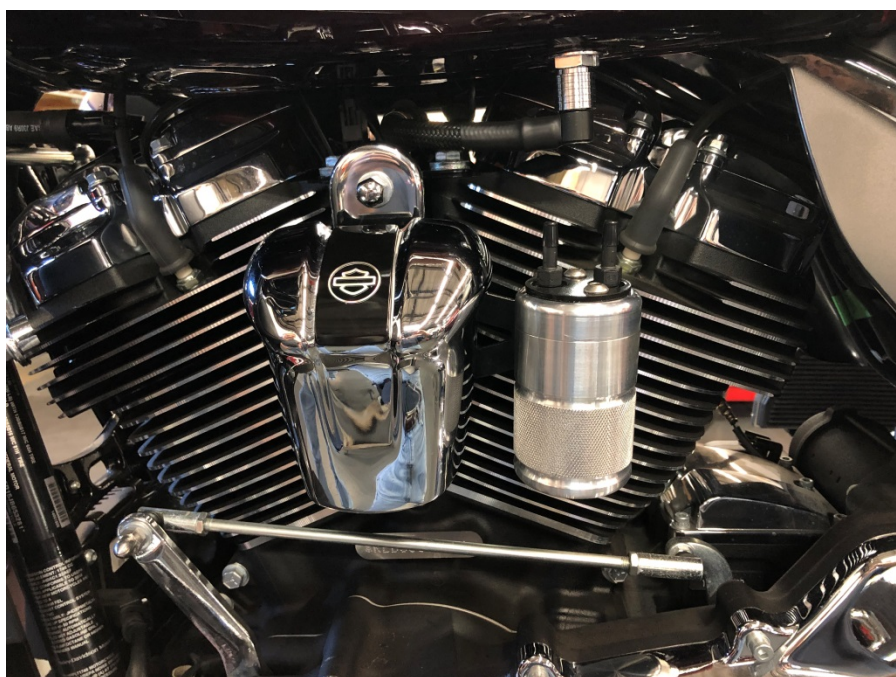
Step 11: Re-assemble horn assembly to motorcycle
