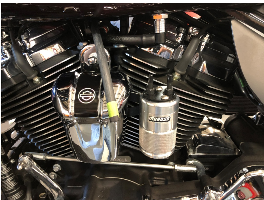
Step 16: Route ¼" end of line with masking tape from right side of motorcycle to left side as shown.
