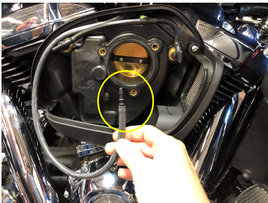
Step 28: Install 3/16" to 3/16" coupling in return line.
