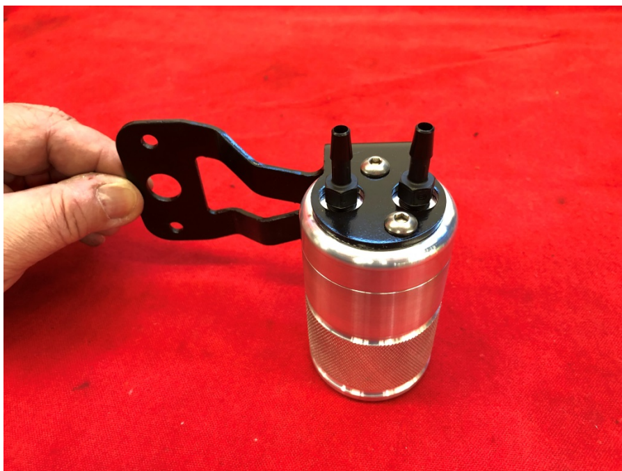
Step 6: Assemble Air oil separator to bracket using (2) \frac{1}{4} -20x.1/2 pan head bolts provided in kit, Install (2) 1/8" NPT x \frac{1}{4} " hose barbs in Air Oil Separator.
