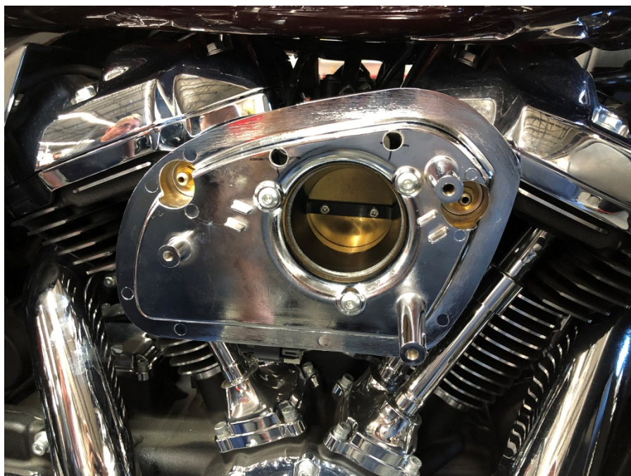
Step 12: Re-assemble air pan to motorcycle.
