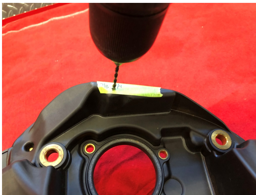
Step 11: Drill centering hole as needed using 1/8" drill bit.
