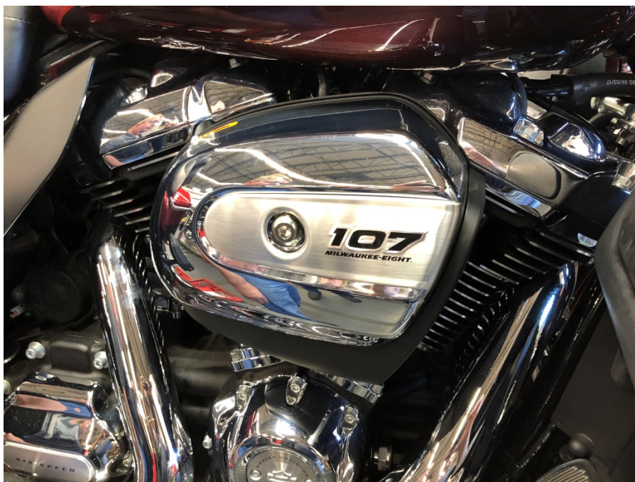
Step 31: Re-install air cleaner cover.
