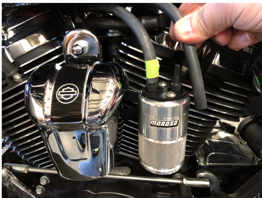
Step 25: Install breather line with masking tape to forward barbed fitting and install return line to rear barbed fitting.
