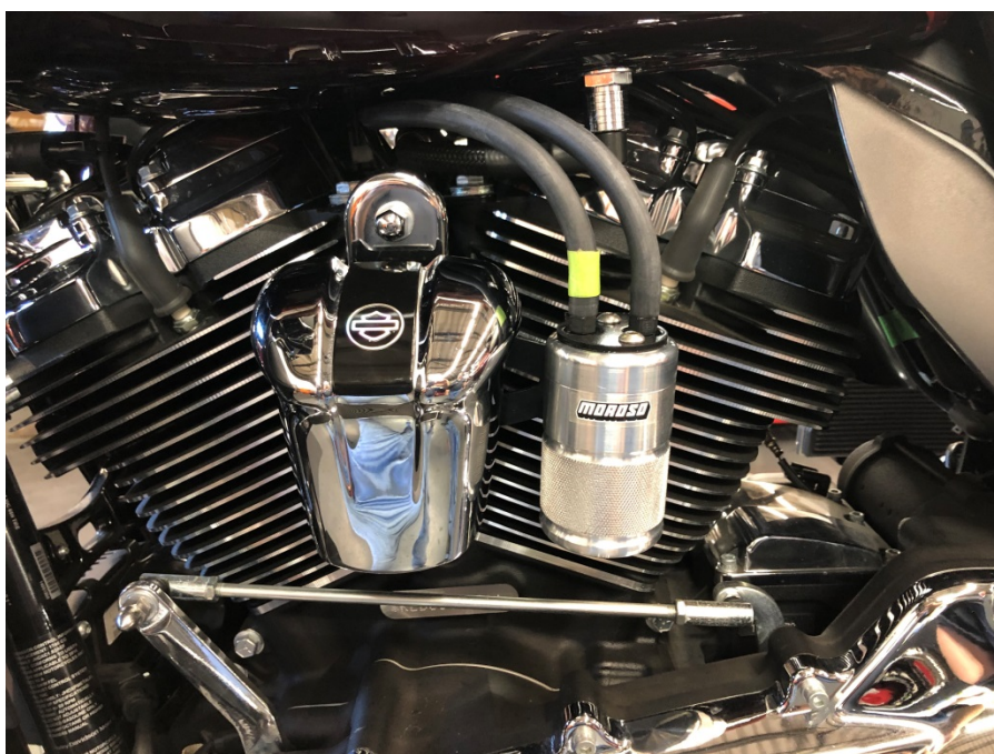
Step 32: Install breather line with masking tape to forward barbed fitting and install return line to rear barbed fitting.
