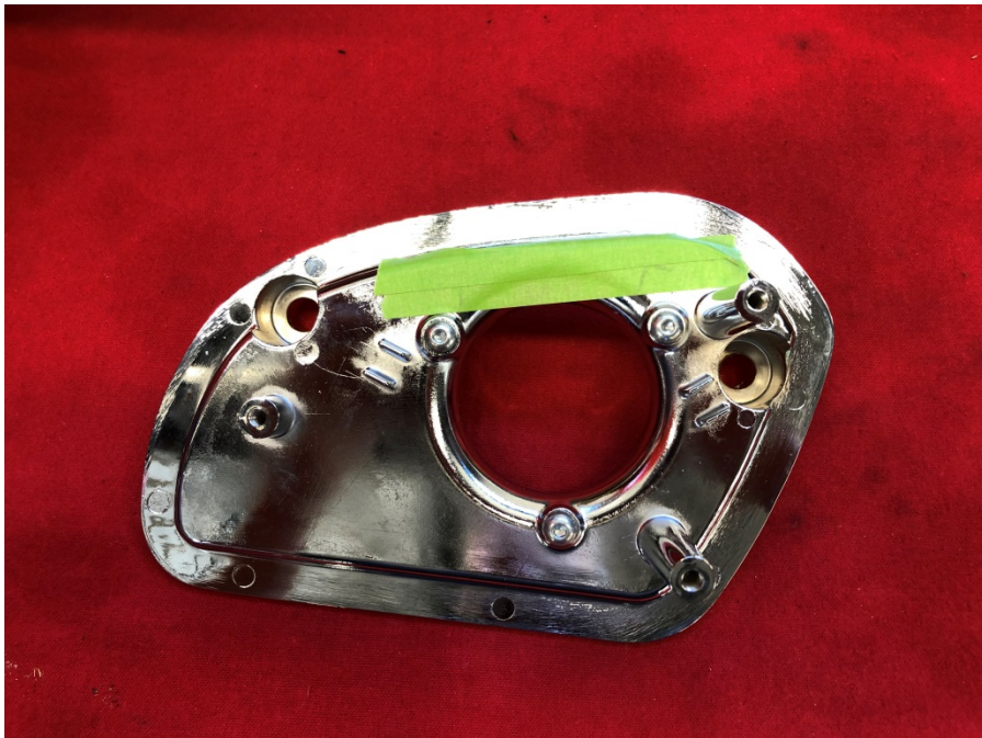
Step 3: Apply masking tape to top of air pan as shown.
