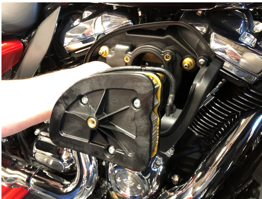
Step 1: Remove air cleaner cover and air cleaner.
