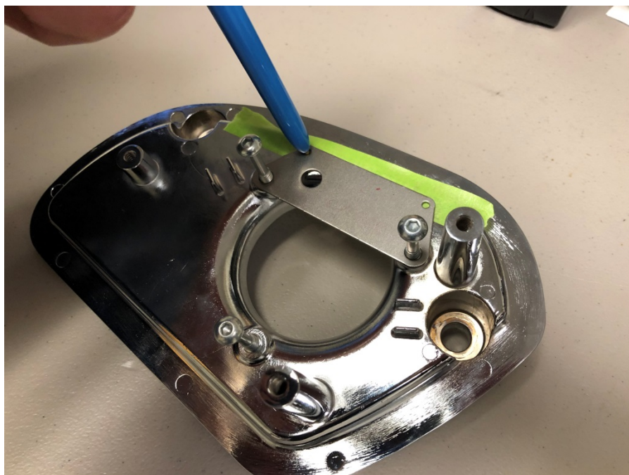
Step 5: Mark center line of holes using pencil / pen or center punch.
