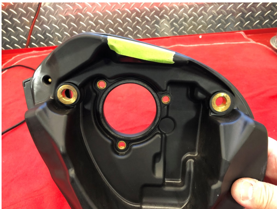
Step 9: Apply masking tape as shown to back side of air pan.
