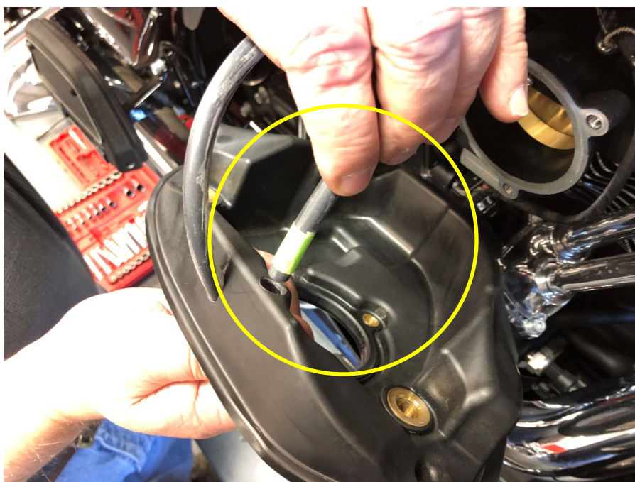
Step 22: Insert line with masking tape through back hole in air pan.
