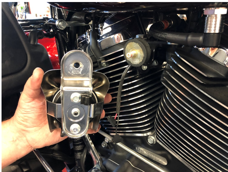
Step 7: Remove horn from motorcycle.
