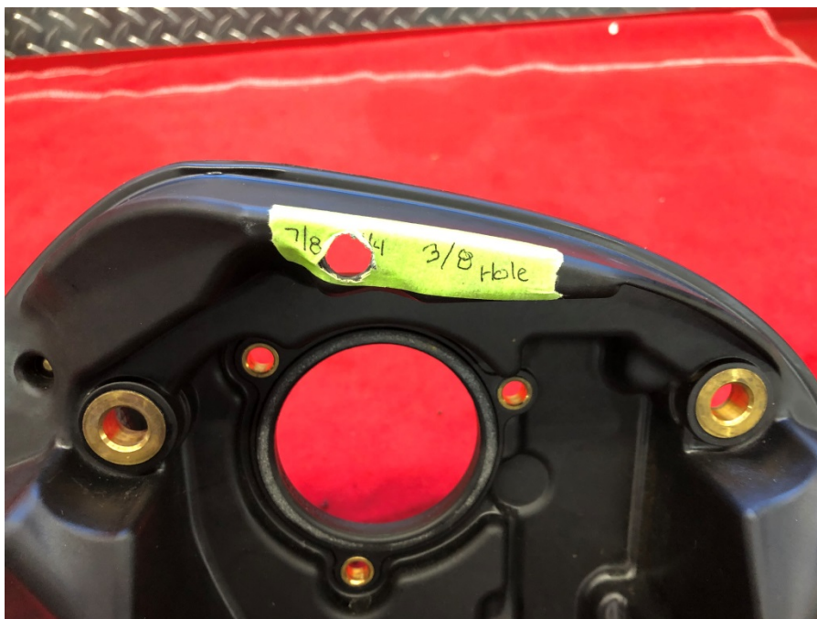
Step 12: Open up 1/8" pilot hole previously drilled with 3/8" drill bit.
