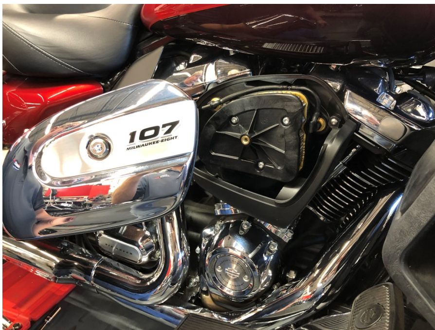
Step 1: Remove air cleaner cover and air cleaner.
