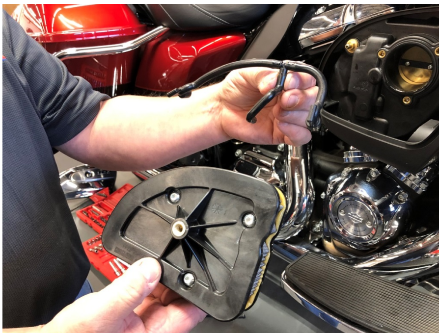
Step 2: Remove breather lines from air cleaner and set aside for future steps.
