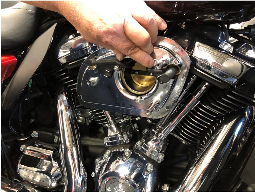
Step 2: Remove breather tubes and air pan.
