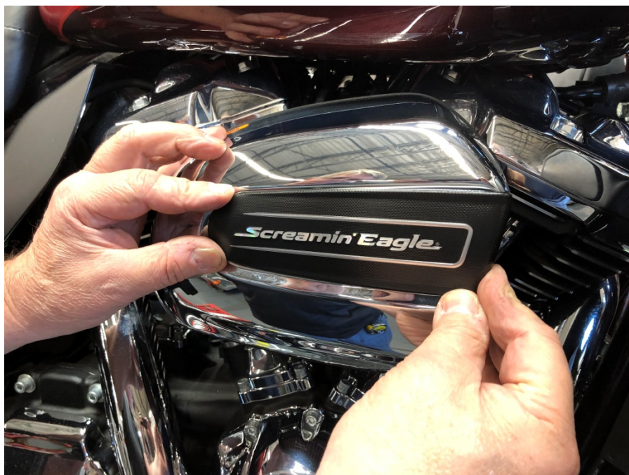
Step 24: Re-install air filter cover.
