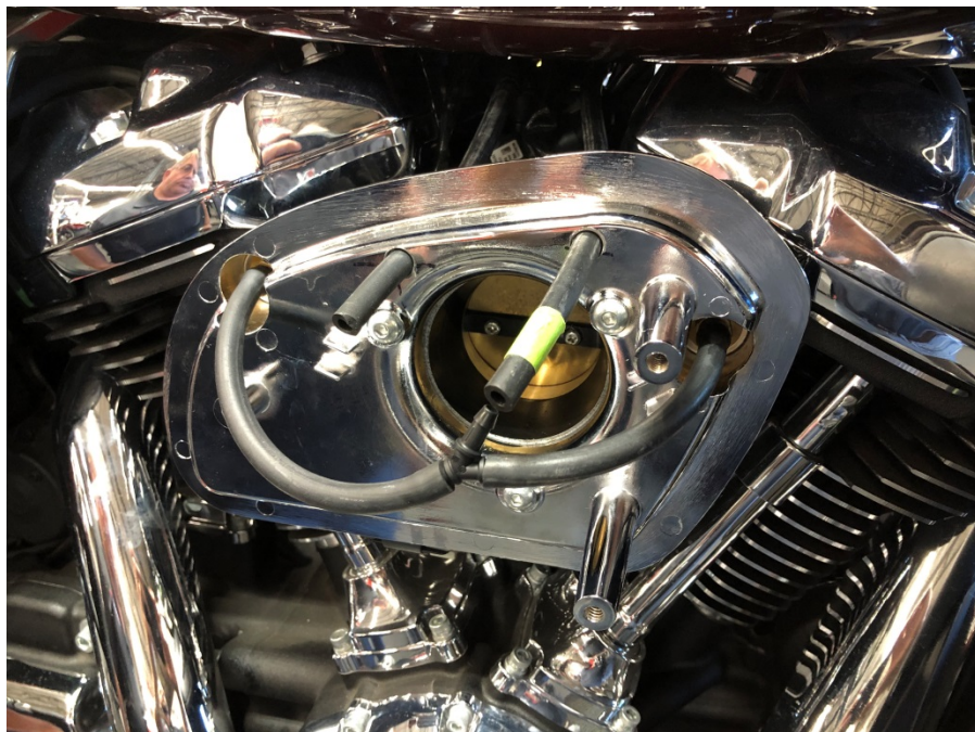
Step 19: Connect line assembled in step 15 to head vent bolts.
