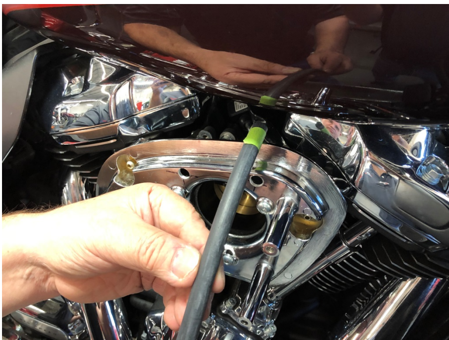
Step 16: Route ¼" end of line with masking tape from right side of motorcycle to left side as shown.
