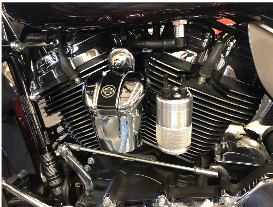
Step 8: Re-assemble horn assembly to motorcycle.
