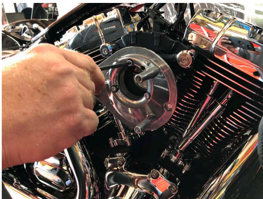
Step 2: Remove air pan.
