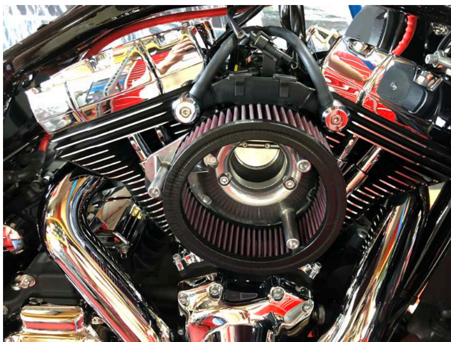
Step 17: Re-install head vent bolts covers, air filter and air filter cover.
