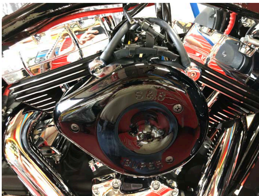
Step 17: Re-install head vent bolts covers, air filter and air filter cover.
