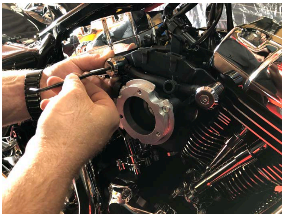
Step 3: Remove Head vent bolt covers.
