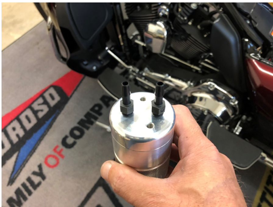
Step 13: Install (2) 1/8" NPT x 1/4" hose barbs in Air Oil Separator.
