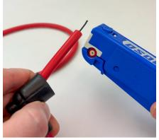
5. Fold the conductor back over the insulation, slip the terminal over the lead and crimp terminal to the wire. (Moroso Crimp Tool; P/N 62268)
