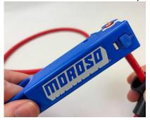
4. Remove the cut insulation and wire stripping tool. Trim any loose strands from the wound conductor; side cutters are best for this.
