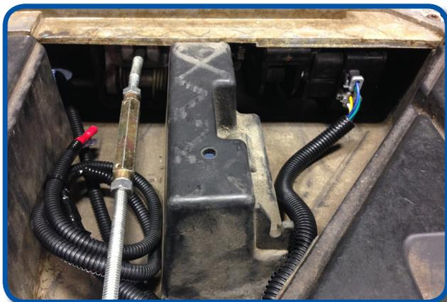
(A) Re-attach brake pedal cover.
