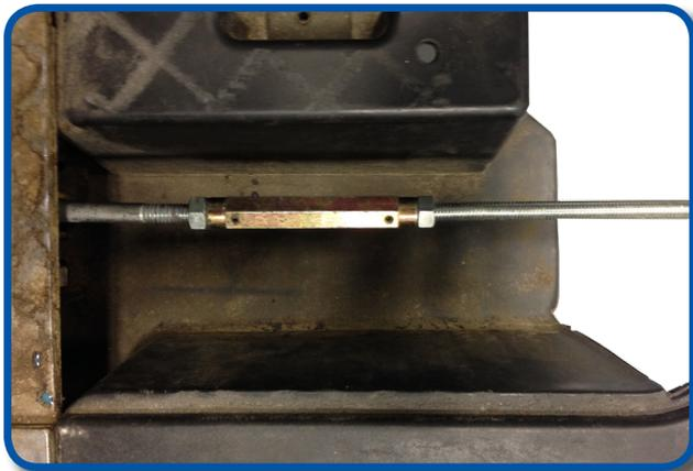
Apply thread locking adhesive to the opposite end of extension rod. Insert opposite end of rod into turnbuckle until threads are visible in the witness hole as shown. Rotate turnbuckle until threads are shown past the witness holes.
