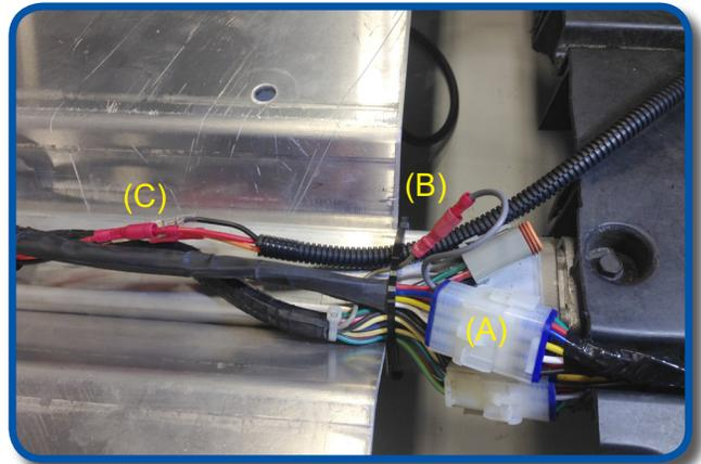
Feed brake pad plugs into pedal box and secure. You can now attach your harness plugs to the brake pad plugs if applicable.
