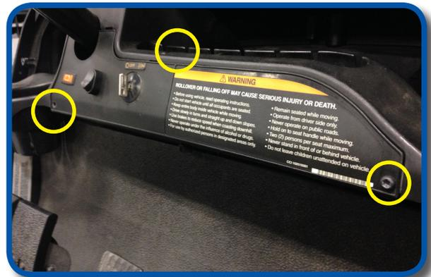
Remove 2 screws and rivet from dash assembly. Retain Hardware.
