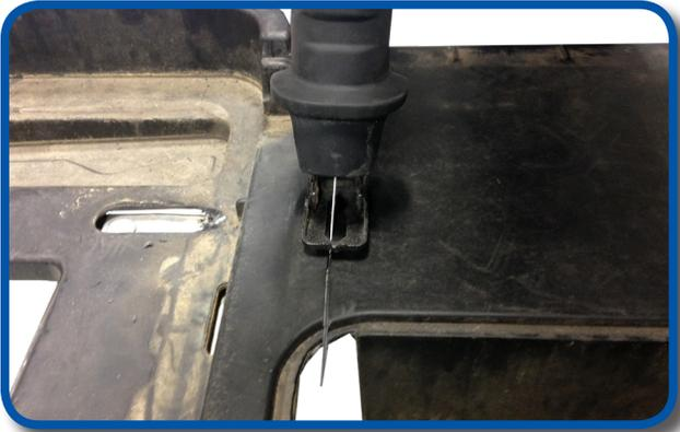
Starting in pedal box, cut back towards frame as shown. **Do not cut into frame.**
