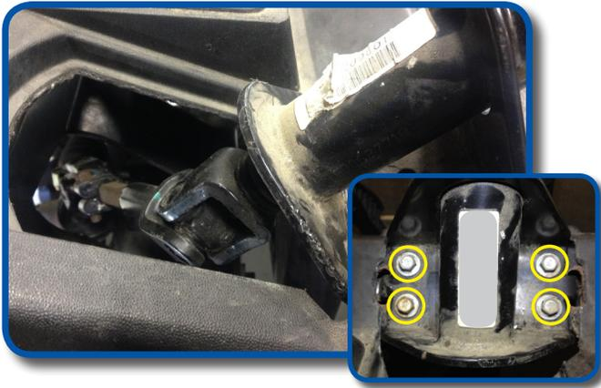
Remove the 4 bolts that attach the steering column to the frame. Retain Hardware.
