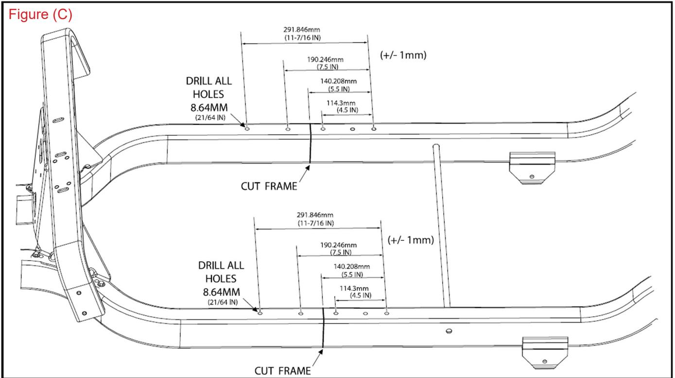
Measure, Mark, Drill, and Cut Frame Rails
