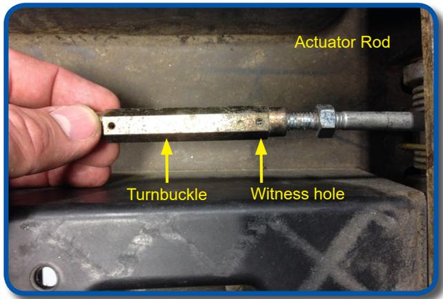
At the brake pedal apply thread locking adhesive to the threads of the actuator rod. Then thread the turnbuckle onto the rod until the threads are visible in the witness hole of the turnbuckle as shown.
