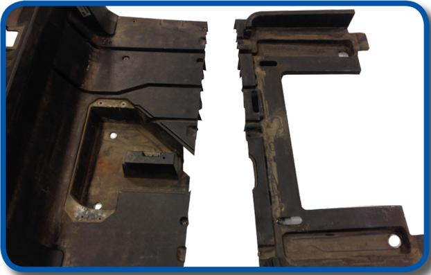
Remove the under body from cart and finish cutting along chalk line where the frame was.
