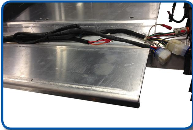
For carts 2008.5 and newer route bucket harness in same "V" channel as factory harness. Excess harness will need to be tied together in channel so 12 pin connector will equal factory 12 pin connector location from previous step.
