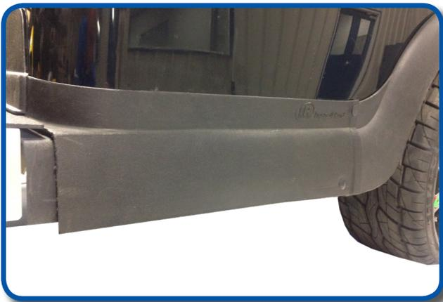
Re-attach rear mat retainer to hold side body panel in place.
