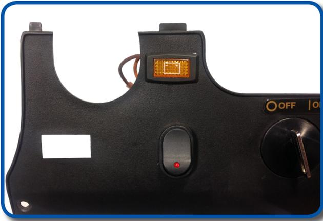
Enlarge the existing battery warning lamp hole for the F-N-R switch. New dimensions should be 1.5" wide x 13/16" tall. Refer to [Figure D](#) if needed.
