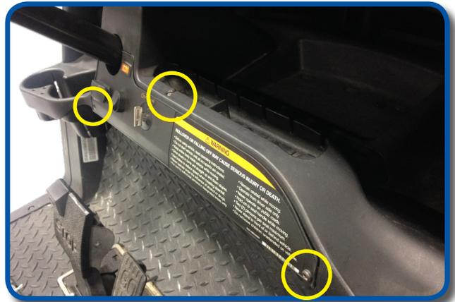
Attach new floormat retainers (from box 2) to floor board using 30mm rivets from Pack #3.
