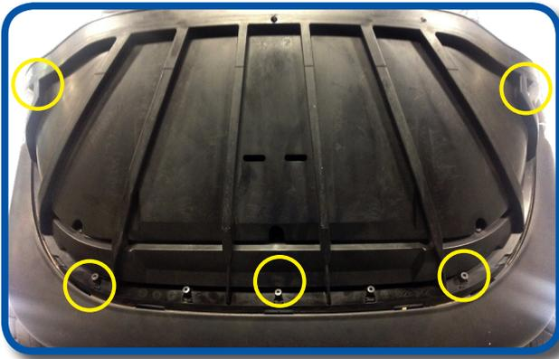
Remove front Brow and Fascia assembly from front under body by removing 5 screws shown and retain.
