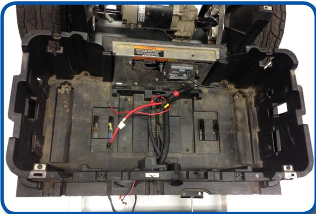
Reattach battery box to the frame using retained hardware from step 28
