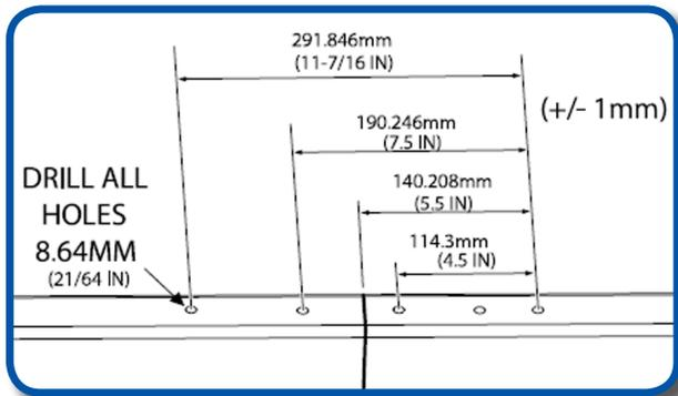
Drill a 21/64 inch hole in the top of the frame only. The bottom will be drilled in a later step to ensure accuracy.
