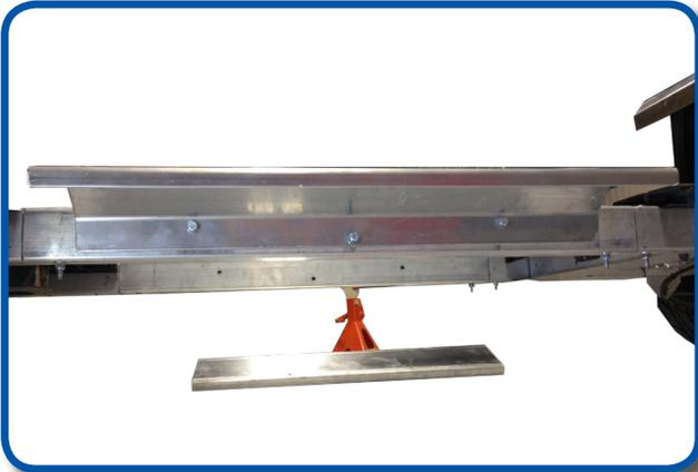
Using the six 8 x 75mm bolts from Pack #2 attach the side supports to the frame. DO NOT push bolt all the way through the frame until next step.
