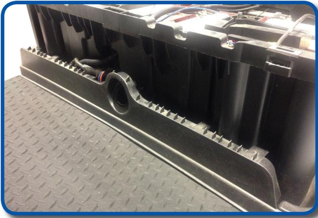
Reattach floor cover plate in three locations using retained hardware and replace charge port cover from steps 17 and 18.
