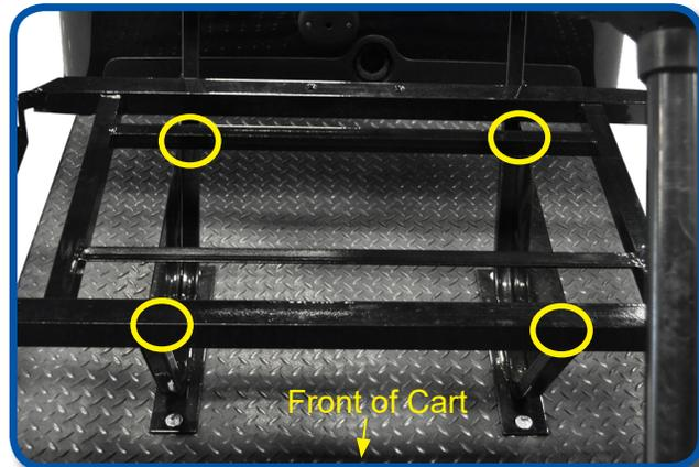
Attach seat support bracket to seat frames using four 8mm x 45mm bolts and hardware from Pack #4. Tighten hardware.
