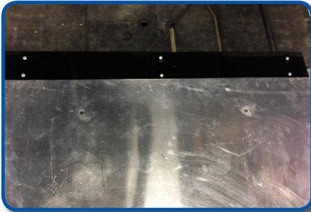
Secure seat frame to floor board using four 8mm x 35mm bolts and hardware from Pack #4. DO NOT tighten until after next step.
