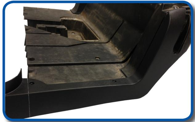
Remove 4 bolts from cross frame and retain all. Slide cross frame off of vehicle frame.
