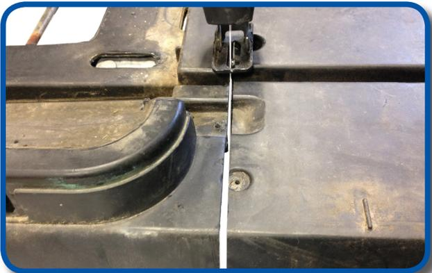
Cut along cut line from outside of passenger side to frame. As shown. **Do not cut frame.**
