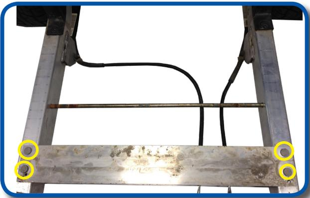
**NOTE:** before cutting frame, support the frame with jack stands or blocks. Be sure cart will not roll once frame has been cut. It's advised to place supports on both sides of cutting location.
