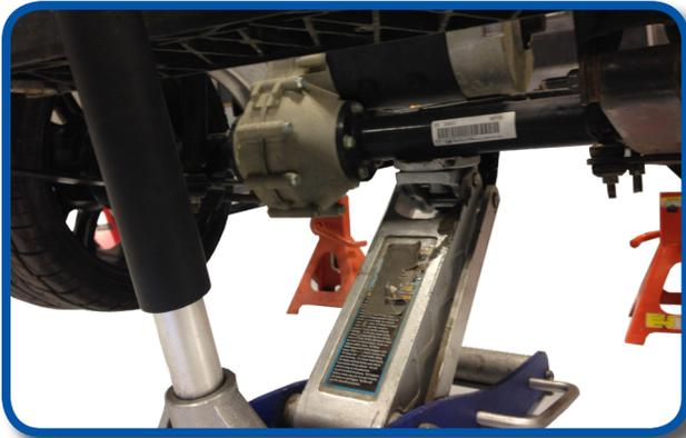
**NOTE:** Using floor jack to support axle raise jack enough to relieve tension on rear shocks.
