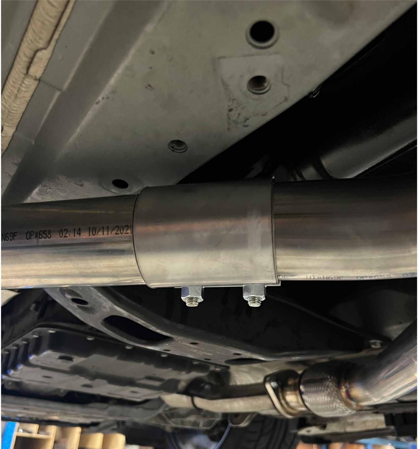
Secure the driver side Y-Pipe leg with included slip clamp
