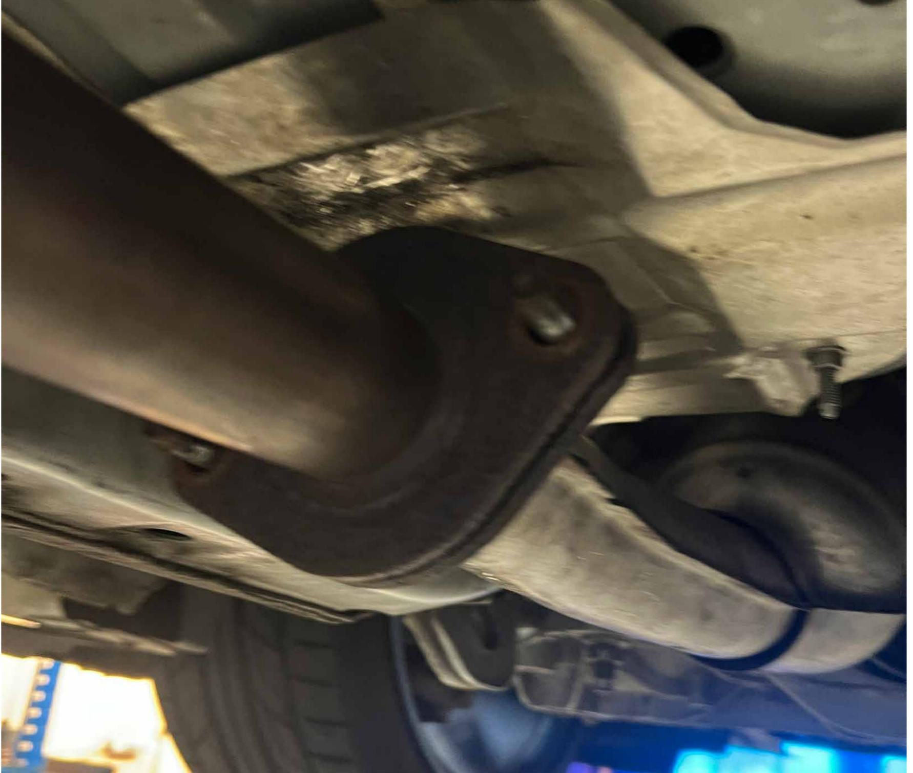
Remove OEM Y-Pipe to downpipe nuts
