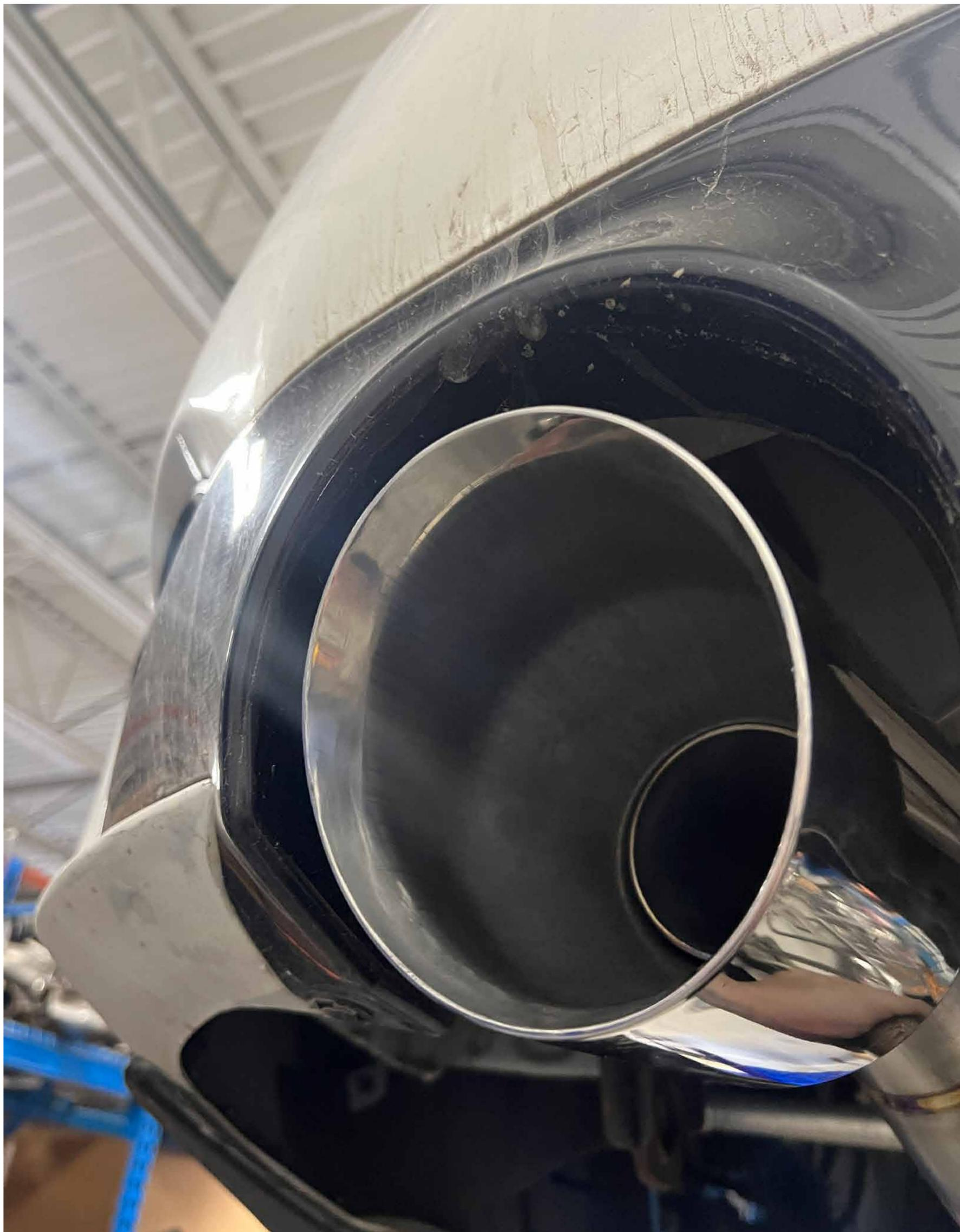
Install tips on both sides, be sure to use included anti-seize on clamp threads
