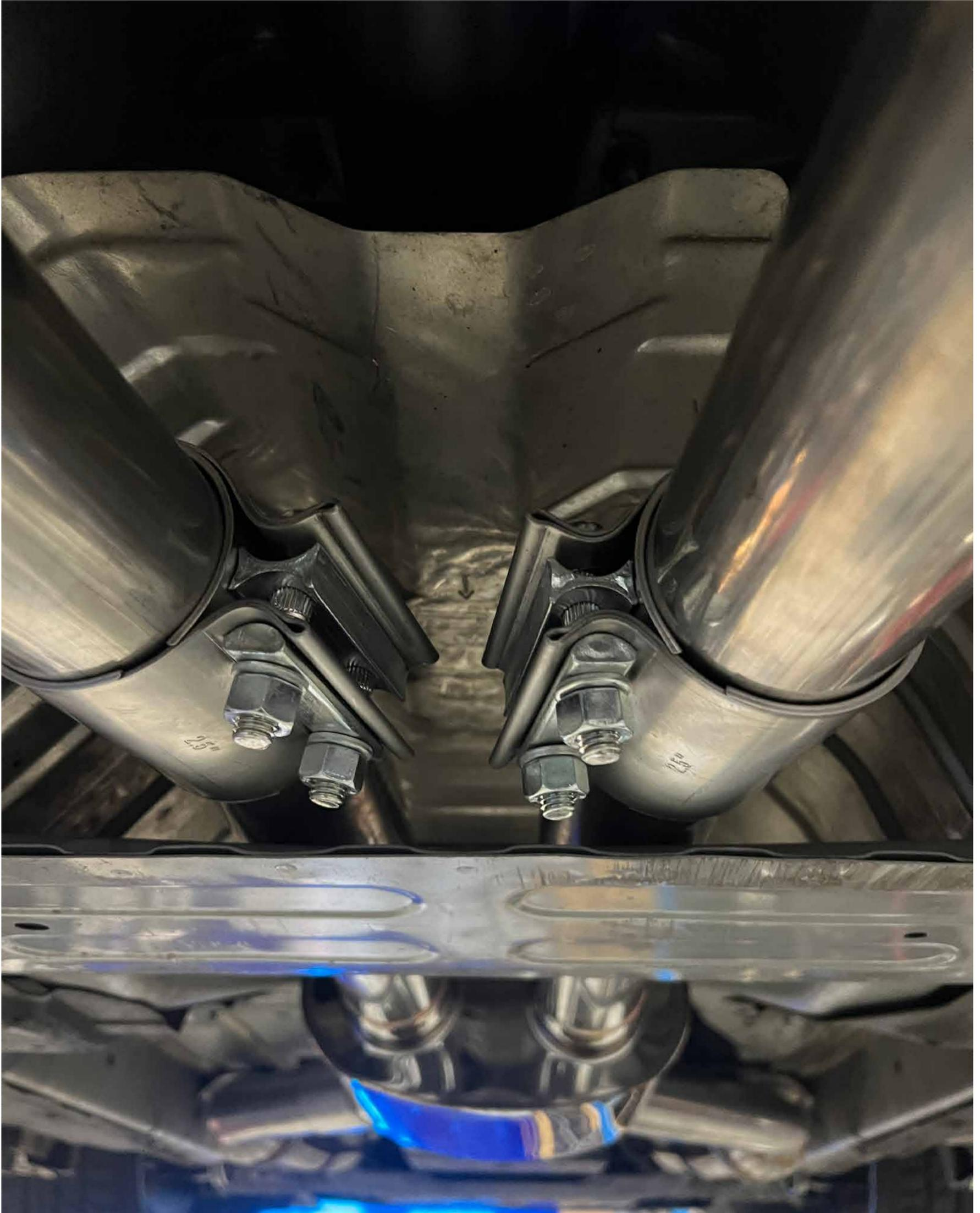
Install slip clamps on both sides of exhaust and tighten
