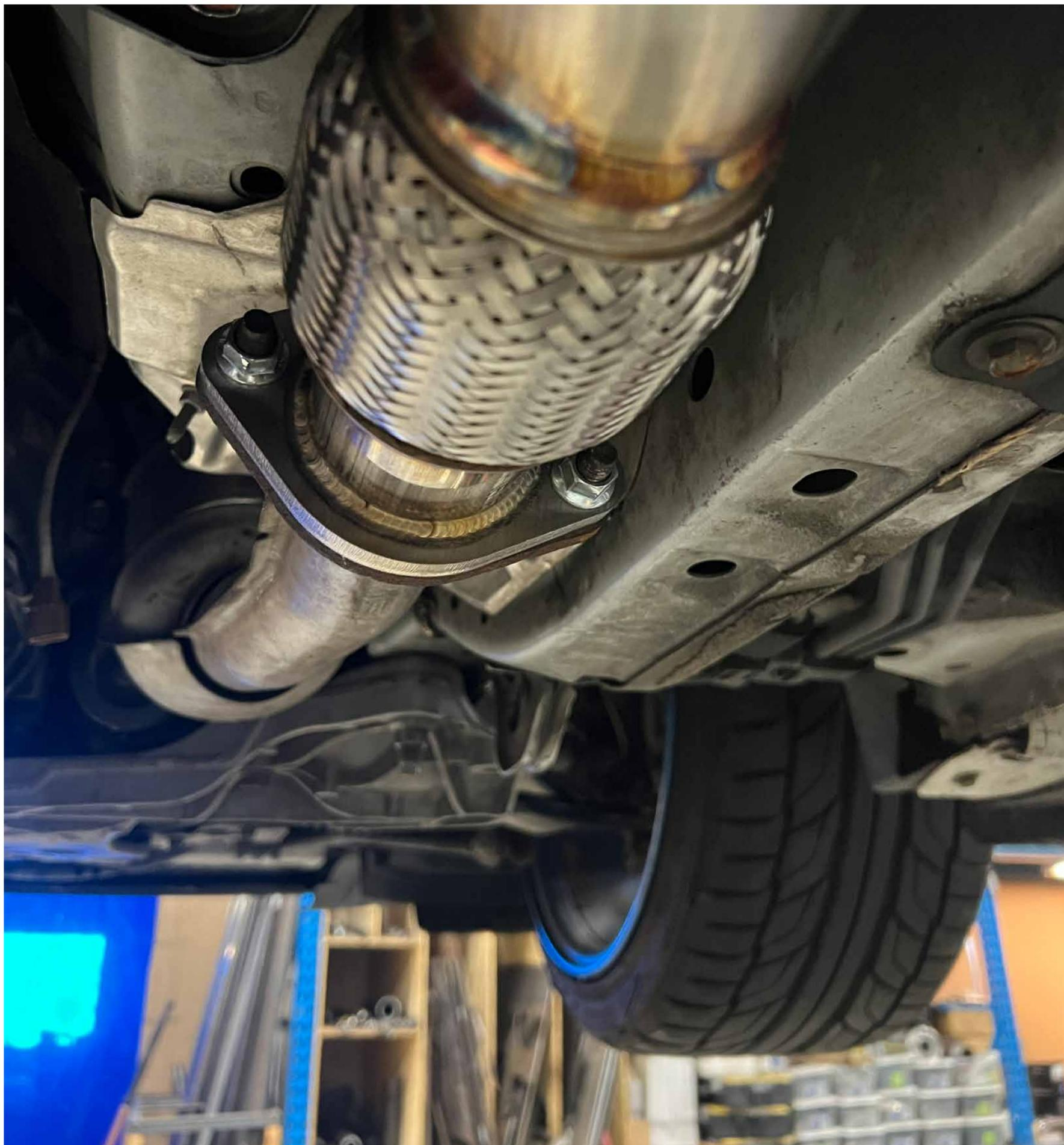
Install MAP Y-Pipe onto the passenger side downpipe and secure it with included hardware. Be sure to use the included downpipe gasket. Reinstall lower support brace.
