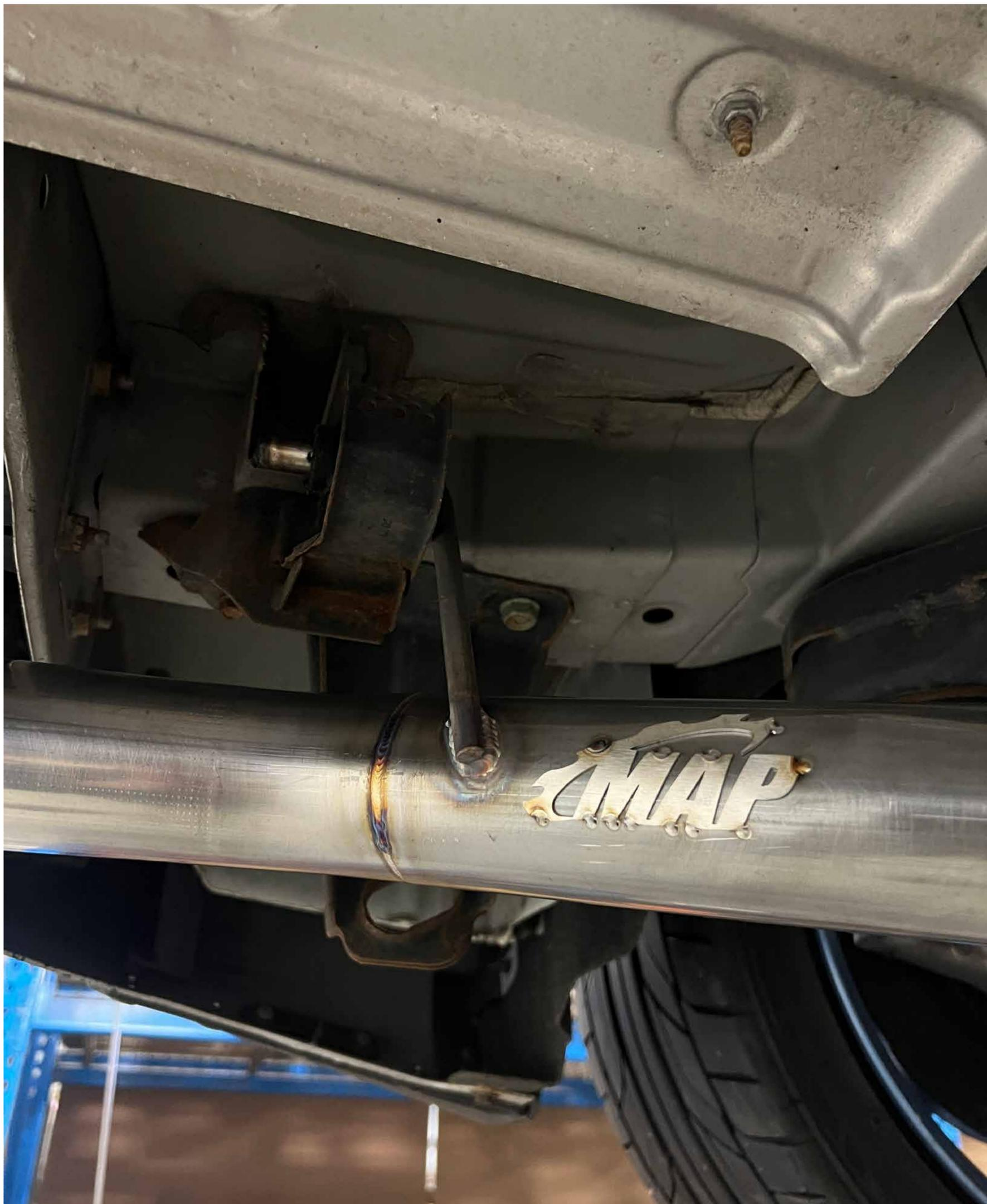
Install rear exhaust section utilizing the oem hangers to hold the exhaust in place
