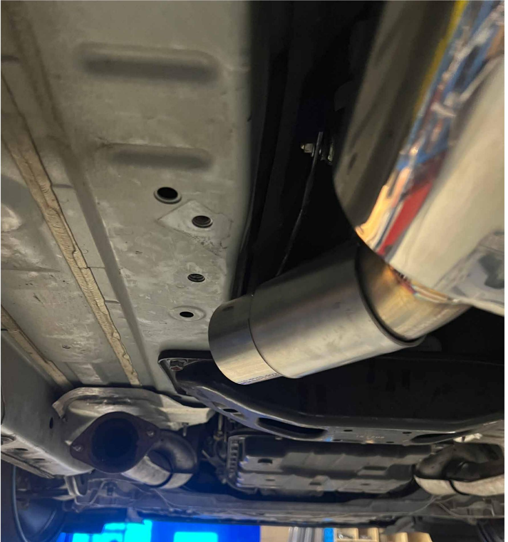
Install driver side Y-Pipe leg onto the drivers side downpipe, install with included gasket and hardware.
