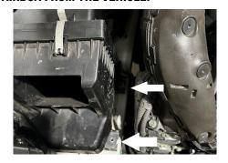
5. INSIDE THE FENDER WELL, REMOVE THE 12MM BOLT SECURING THE INTAKE BRACKET TO THE CHASSIS OF THE VEHICLE. YOU MAY NEED TO PARTIALLY REMOVE THE PLASTIC UNDER TRAY FOR ACCESS.
