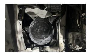
10. ADJUST THE INTAKE PIPE AS NEEDED FOR THE FILTER TO CLEAR THE HEADLIGHT AND SPLASH SHIELD. TIGHTEN THE MOUNTING BOLT AND INTAKE CLAMPS ONCE INTAKE IS POSITIONED CORRECTLY.
