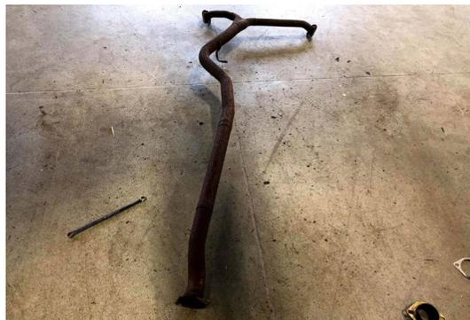
**6. INSTALL NEW MAP MIDPIPE, SECURING IT WILL INCLUDED HARDWARE AND GASKETS, REINSTALL RUBBER HANGERS**
