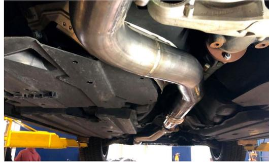
**11. TIGHTEN V BAND CLAMP AND BOTH SLIP CLAMPS**
