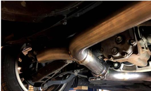
**8. INSTALL MAP MUFFLERS IN PLACE WITH RUBBER HANGERS**
