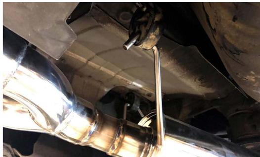
**9. INSTALL SLIP CLAMPS OVER MUFFLERS AND Y PIPE, KEEPING THEM LOOSE**
