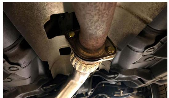
**7. INSTALL NEW MAP Y PIPE, KEEPING THE V BAND LOOSE**
