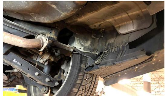
**4. REMOVE 2 BOLTS SECURING YOUR STOCK Y PIPE TO YOUR DOWNPIPE**
