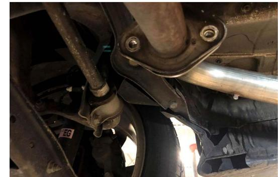
**3. REMOVE RUBBER HANGERS HOLDING THE MUFFLERS TO THE VEHICLE (2 PER SIDE) SET THE MUFFLERS ASIDE**
