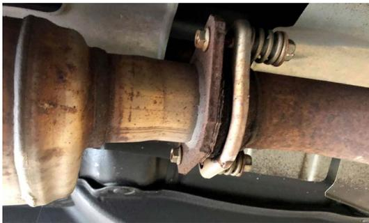
**5. REMOVE RUBBER HANGER SECURING STOCK Y PIPE. SET YOUR FACTORY Y PIPE TO THE SIDE**
