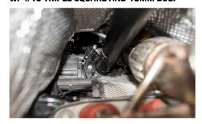
THEN 8MM ALLEN NUTS FOR PASSENGER FRONT AXLE SHIELD
