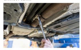
11. REMOVE 02 SENSOR AND UNPLUG COMPLETELY
