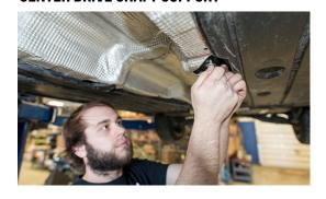
20. REINSTALL HEAT SHIELDS - DRIVE SHAFT W/ #10 TRIPLE SQUARE AND 16MM BOLT
