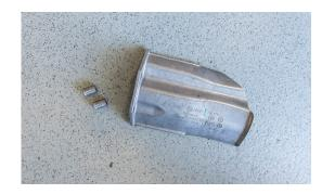
4. REMOVE 16MM BOLT HOLDING DRIVE SHAFT HEAT SHIELD
