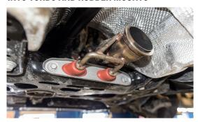
16. TIGHTEN V-BAND CLAMP FULLY TO TOP OF DOWNPIPE AT THE TURBO
