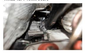
19. REINSTALL FOUR 13MM BOLTS HOLDING CENTER DRIVE SHAFT SUPPORT
