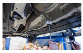
8. MOVE DRIVESHAFT OUT OF THE WAY
