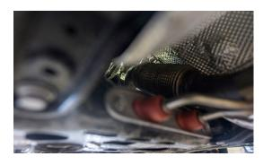
10. LOOSEN TWO 13MM NUTS FROM THE EXHAUST CLAMP
