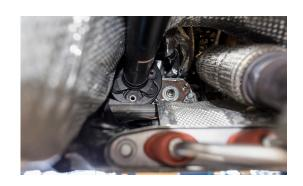
9.REMOVE TWO 13MM NUTS FROM THE DOWNPIPE SUPPORT BRACKET
