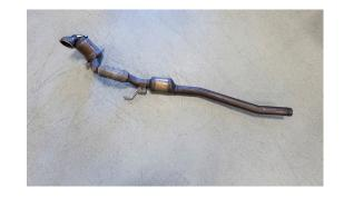
15. INSTALL FRONT SECTION OF MAP DOWNPIPE INTO TURBO AND RUBBER MOUNTS
