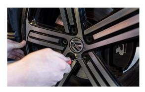
2. REMOVE PASSENGER FRONT WHEEL - 17MM
