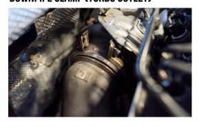
13. PULL DOWNPIPE TOWARDS THE REAR OF THE CAR TO REMOVE FROM RUBBER MOUNTS
