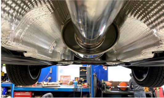
**9. INSTALL MUFFLER SECTION WITH THE OEM HANGER AND MAP HANGER (AS PICTURED)
