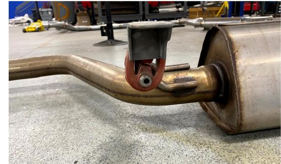
**7. INSTALL THE REAR Y PIPE ONTO THE CAR
