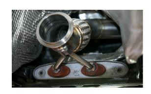
15. ATTACH AND TIGHTEN V-BAND CLAMP TO STRAIGHT DOWNPIPE SECTION
