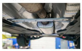
6. REMOVE THE TWO 13MM NUTS FOR THE EXHAUST SLIP JOINT
