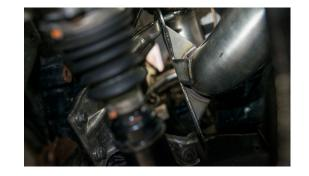
10. START THE TWO 13MM BOLTS FOR SUPPORT BRACKET BUT DO NOT TIGHTEN
