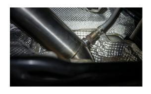
12. TIGHTEN THE V-BAND CLAMP TO TOP OF DOWNPIPE AT TURBO
