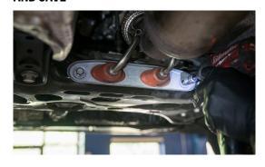
8. REMOVE THE OEM DOWNPIPE FULLY
