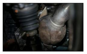
5. REMOVE FOUR 13MM BOLTS FOR THE EXHAUST SUPPORT BRACE
