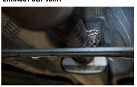
7. REMOVE THE DOWNPIPE HANGER BRACKET AND SAVE
