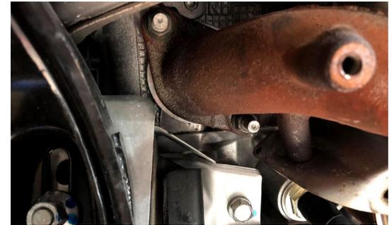
**6. REMOVE FACTORY MANIFOLD FROM THE VEHICLE**
