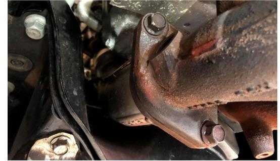
**4. REMOVE 2 BOLTS SECURING FACTORY MANIFOLD TO YOUR UP-PIPE**
