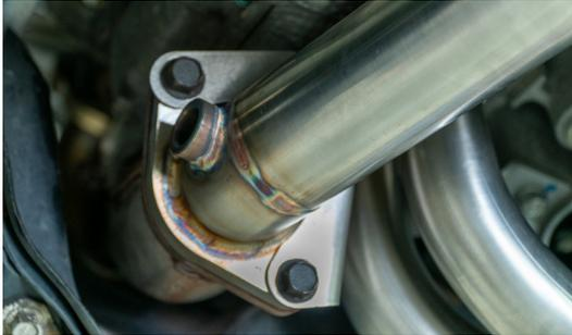
**9. REINSTALL 6 14MM NUTS SECURING MAP ELH TO THE ENGINE**
