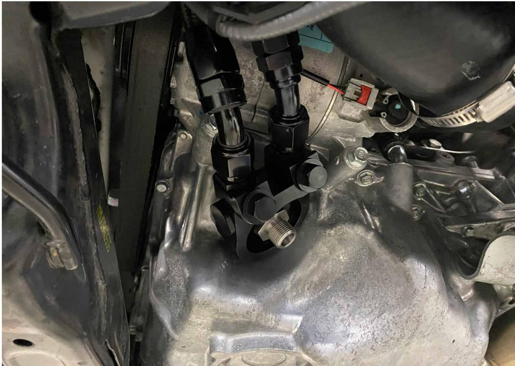
Thread AN Lines onto the oil cooler, longer line goes on drivers side and shorter line will go on passenger. Route as pictured and thread onto oil sandwich plate, once all lines are in place, tighten all fittings and hose ends.
