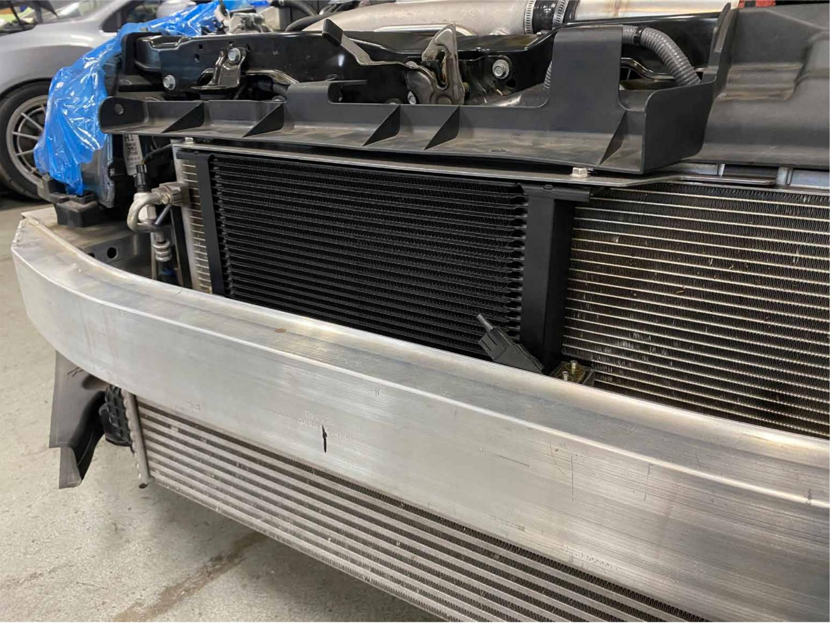
Next, attach MAP FK8 Type R oil cooler to the vehicle by securing it to the radiator condenser, using the 4 10mm bolts you removed earlier.
