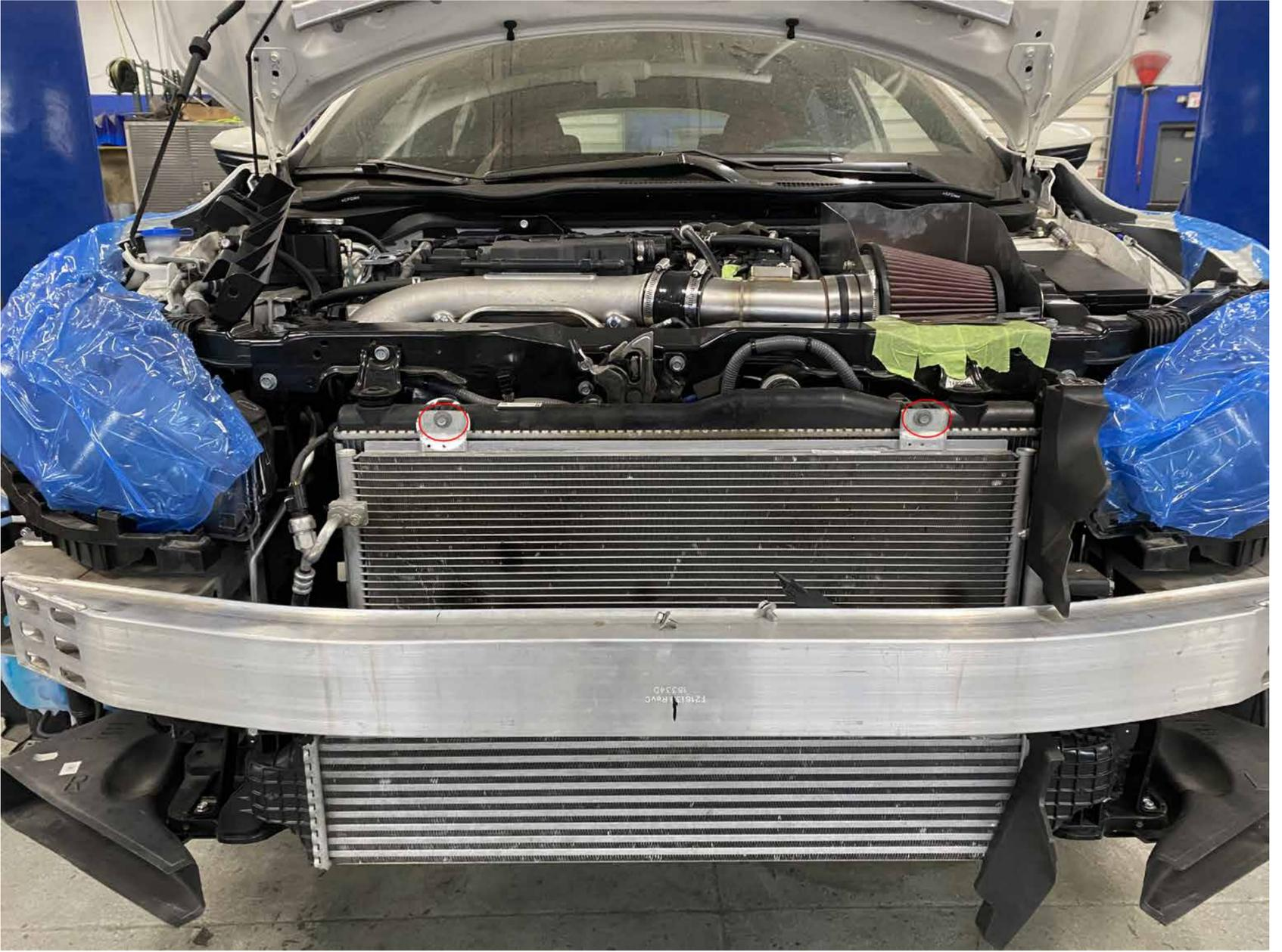
Remove 4 bolts holding AC condenser
