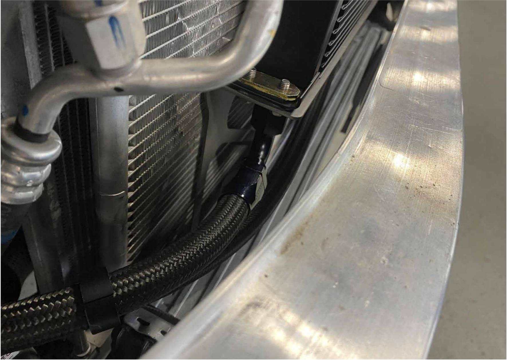
Install included oil sandwich, clock the inlet and outlet as pictured. Tighten to (ftlbs) reinstall oil filter when your finished
