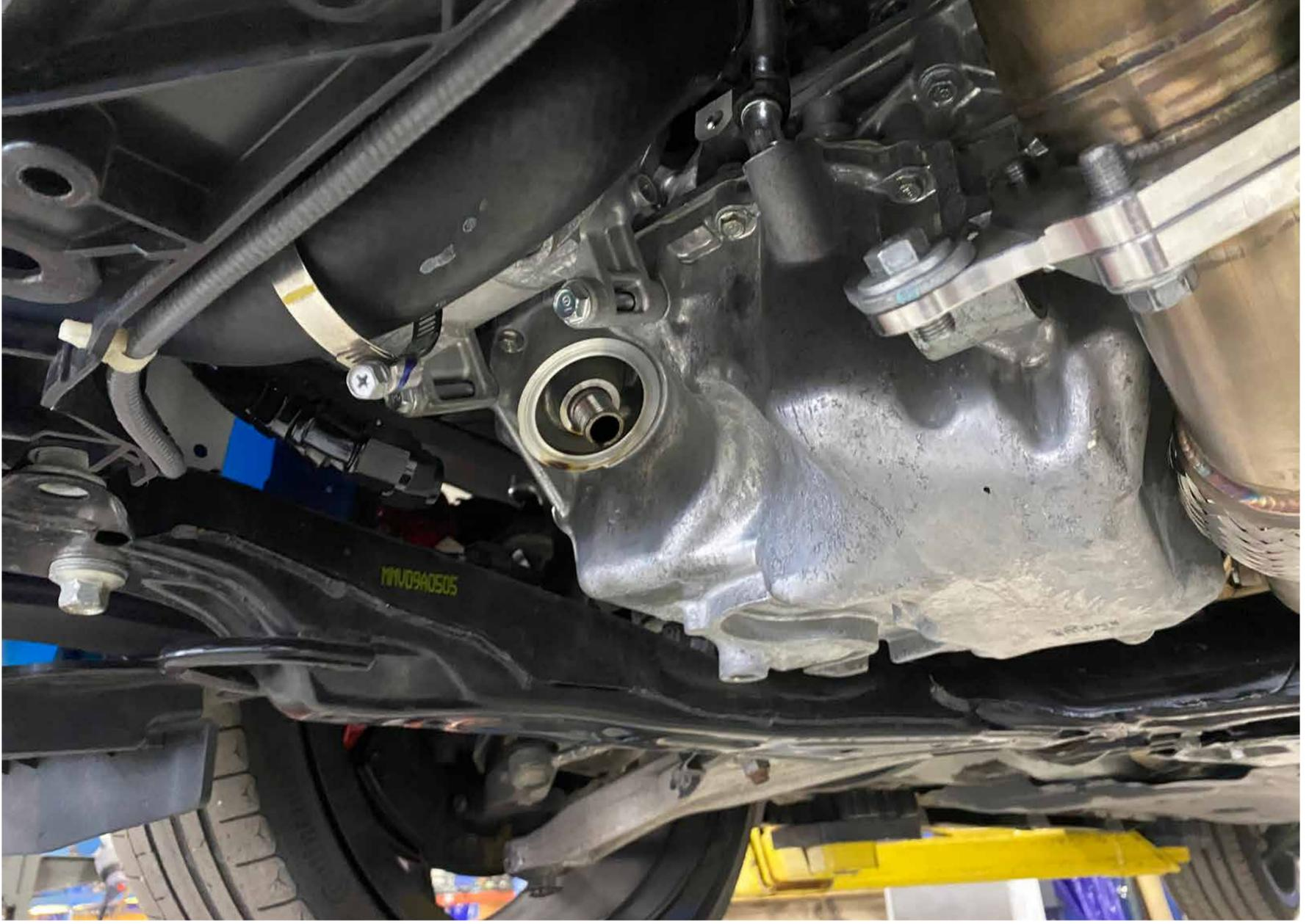
Remove engine oil filter
