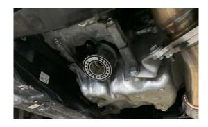
11A-D. INSTALL LOWER HALF OF SANDWICH PLATE, USING INCLUDED HARDWARE (5MM AL-Len) to secure the 2 halves together. Install oil filter adapter to the end of the Sandwich plate, this allows you to thread your oil filter onto the sandwich plate. Ensure the black orb caps are installed in the bottom (as pictured) these seal the 5MM allen head bolts you installed from leaking and are not just for looks (18MM)
