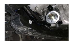
13A-D. ROUTE SHORT LINE FROM PASSENGER SIDE OF OIL COOLER TO THE TOP HALF OF THE OIL COOLER, TIGHTEN BOTH HOSE ENDS AND ORB FITTINGS
