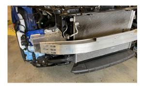
6A-C. ASSEMBLE OIL COOLER AND BRACKET AS PICTURED, LEAVING THE OUTER BOTTOM 2 HOLES WITHOUT BOLTS AS THIS WILL BE USED LATER TO SECURE COOLER LINES. THREAD THE TWO M22TO-10AN ADAPTERS INTO THE TOP OF THE OIL COOLER AND TIGHTEN.
