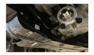
12A-D. ROUTE THE LONGER LINE FROM THE DRIVERS SIDE OF THE OIL COOLER TO THE LOWER HALF OF THE SANDWICH PLATE, SECURE WITH BLACK P CLAMPS SUPPLIED, THESE WILL MOUNT TO THE OIL COOLER IN THE HOLES YOU LEFT OPEN EARLIER. ENSURE THE HOSE ENDS ARE TIGHT AND ORB FITTINGS ARE TIGHT (-10AN)
