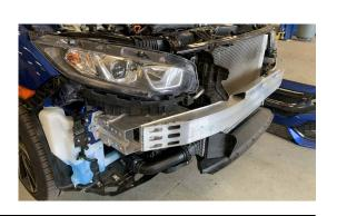
5A-C. REMOVE PLASTIC SHROUD PICTURED, THIS WILL ALLOW YOU TO ROUTE THE COOLER LINES(REMOVE CLIPS AND PULL) THEN REINSTALL THE HEADLIGHT (5 10MM BOLTS)
