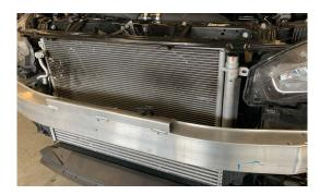
8A-E. ATTACH COOLER ASSEMBLY TO VEHICLE BY REUSING THE BOLTS YOU REMOVED FROM THE AC CONDENSER, SECURING BOTH AC CONDENSER AND OIL COOLER FROM THE SAME MOUNT
