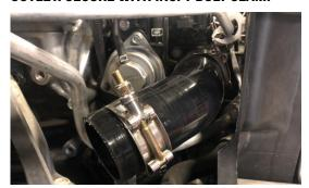
19. INSTALL PICTURED HOT SIDE CHARGE PIPE INTO THE ELBOW COUPLER, SECURE WITH CLAMPS LOOSELY
