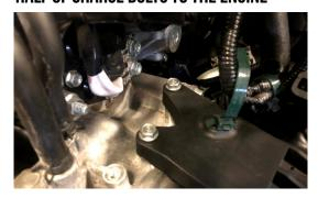
6. REMOVE THE VACUUM LINE AND THE 2 SENSOR CONNECTORS ON THE UPPER CHARGE PIPE
