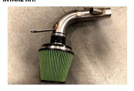
14A. INSTALL INTAKE COUPER AND PIPE WITH AIR FILTER ONTO TURBO INLET, SECURE WITH INCLUDED CLAMPS
