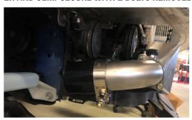
21. SLIDE THE UPPER AND LOWER PIPES TOGETHER AND SECURE WITH THE COUPLER AND CLAMPS.
