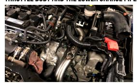
11. GO BACK TO YOUR OEM CHARGE PIPES AND REMOVE THE IAT SENSOR AND PRESSURE SENSOR FROM THE CHARGE PIPE.
