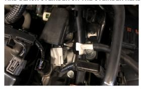
17. REMOVE HOTSIDE CHARGE PIPES BY RE-MOVING CLAMP SECURING TO TURBO OUTLET AND 2 BOLTS FROM INTERCOOLER INLET, THEN ROTATE CHARGE PIPE OUT THE BOTTOM OF THE BUMPER
