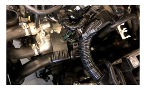
7. LOOSEN CLAMP HOLDING THE COUPLER ON THE UPPER CHARGE PIPE TO THE THROTTLE BODY.
