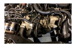
3. REMOVE 2 10MM BOLTS SECURING LOWER CHARGE PIPE ONTO INTERCOOLER - THIS STEP MAY VARY IF USING MAP INTERCOOLER, YOU WILL REMOVE THE CLAMP, COUPLER AND PIPE INSTEAD
