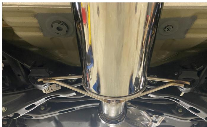
**10. INSTALL SLIP CLAMP ONTO FRONT RESONATED SECTION**
