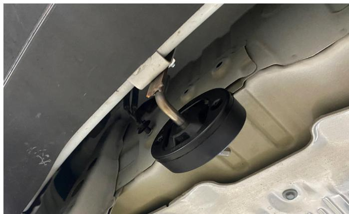
**9. INSTALL MUFFLER SECTION ONTO RUBBER HANGERS**
