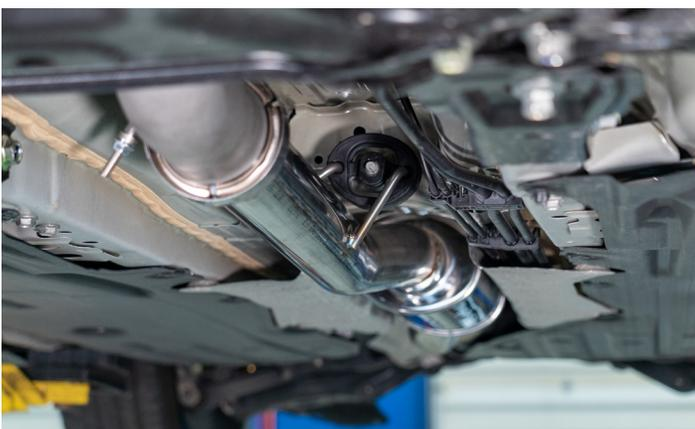
**7. INSTALL THE FRONT RESONATED SECTION ONTO THE MIDPIPE FRONT CONNECTION SECURING IT LOOSELY. BE SURE THE RUBBER HANGER IS SECURED ONTO ITS HANGER OFF THE BODY**
