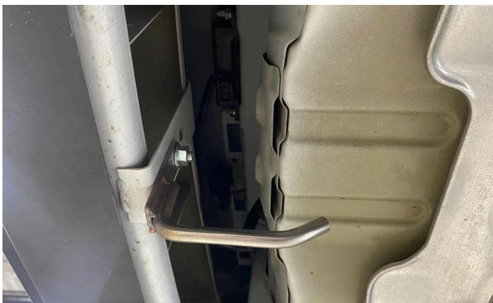
**8B. INSTALL ONE OF OUTER OEM MUFFLER RUBBER HANGERS, INSTALLED AS PICTURED**
