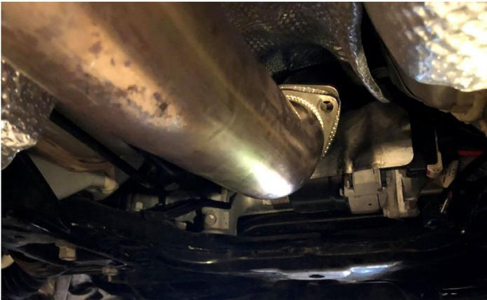
**4. REMOVE REMAINING RUBBER HANGER AND REMOVE THE REST OF THE EXHAUST FROM THE CAR**
