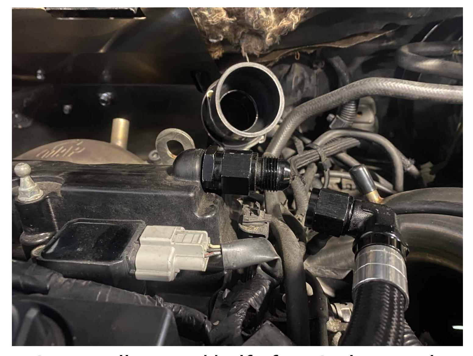
8.P2. install second half of MAP plastic valve cover fitting by threading it on to the fitting you installed on step P1. snug the 2 halves together
