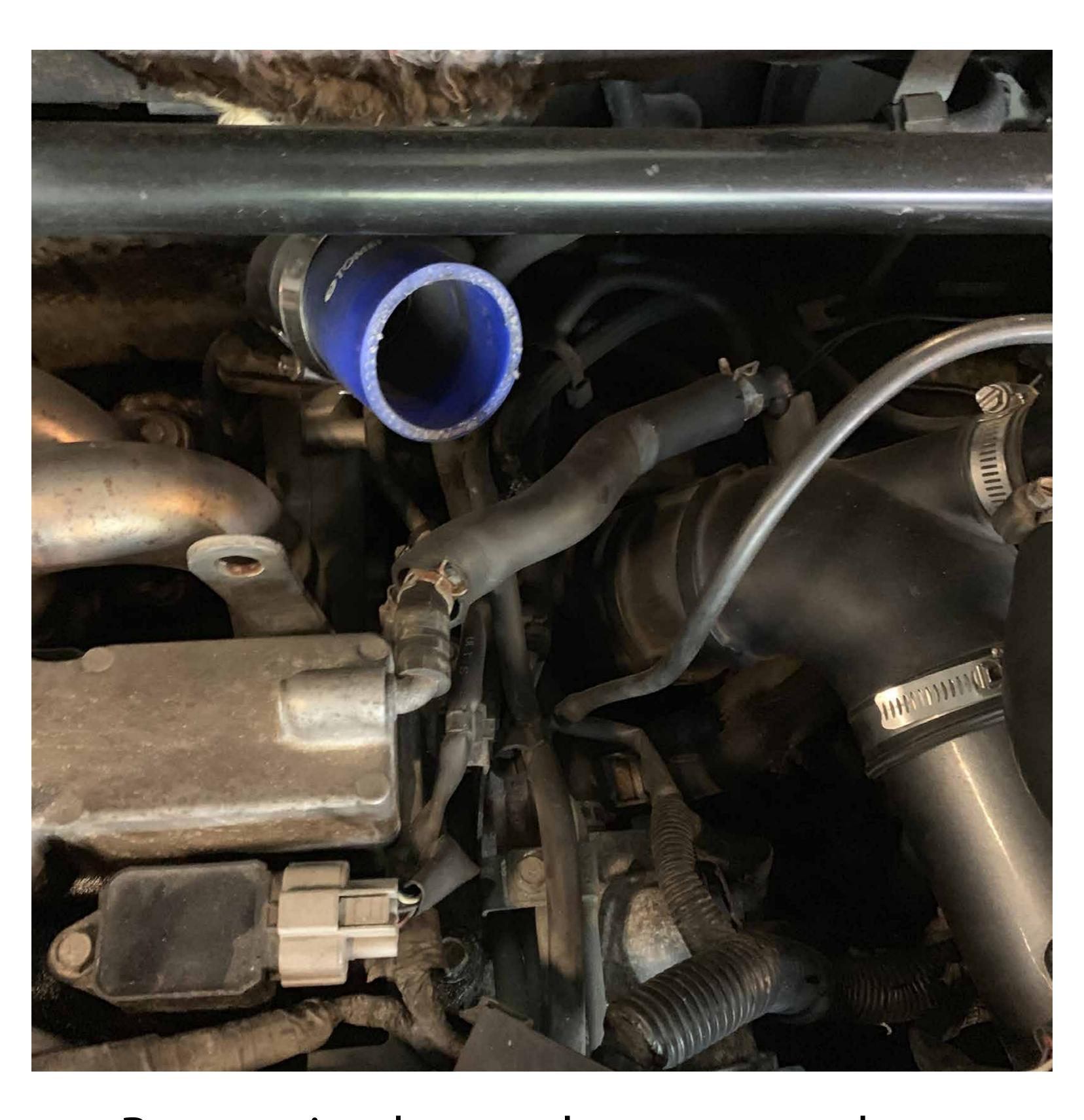
Remove intake to valve cover pcv hose
