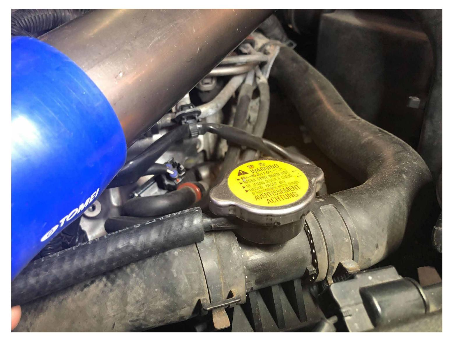
A-B - Route and attach AN lines as pictured, be sure to cap the open vacuum port on intake manifold and intake with included caps
