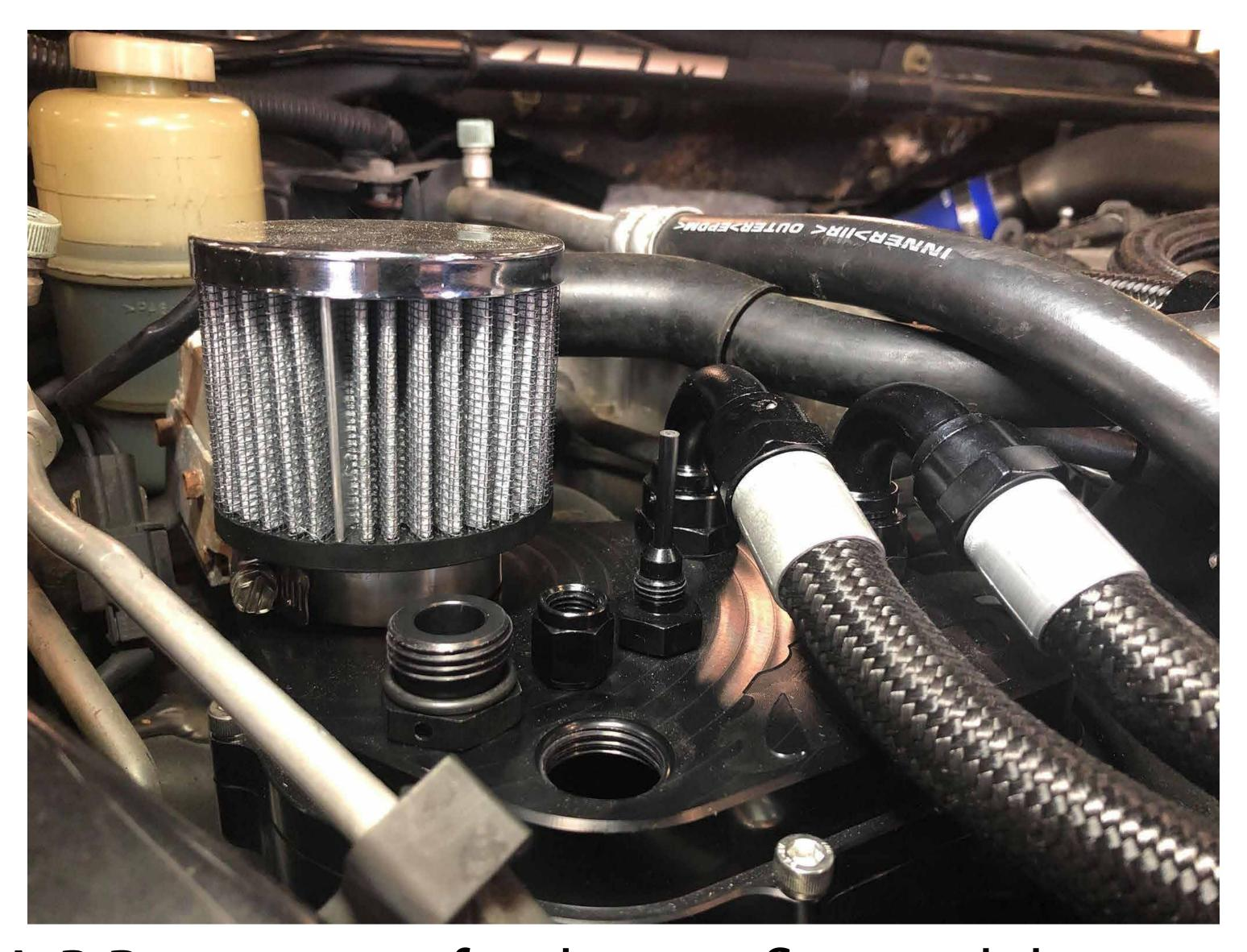
A-B Remove cap for the overflow and the overflow level indicator, fill until bobber reaches half full, reinstall cap
