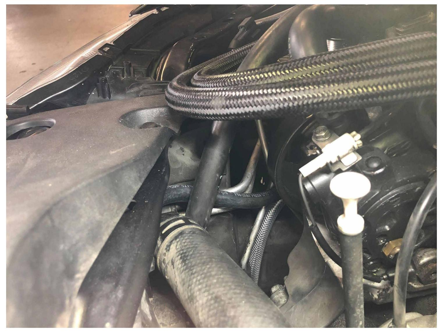
A-B - Run rubber coolant overflow line to radiator
