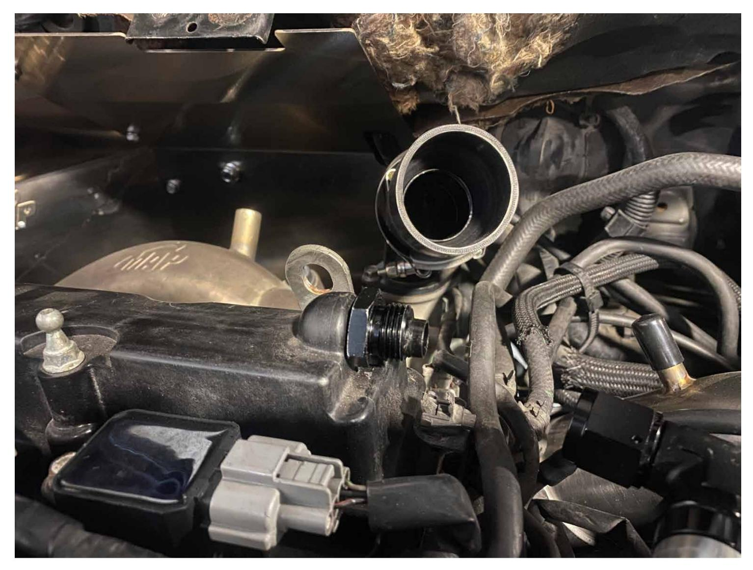
8.P1. install one half of the included MAP plastic valve cover fitting onto the valve cover as pictured. It should fit snugly on the factory barb
