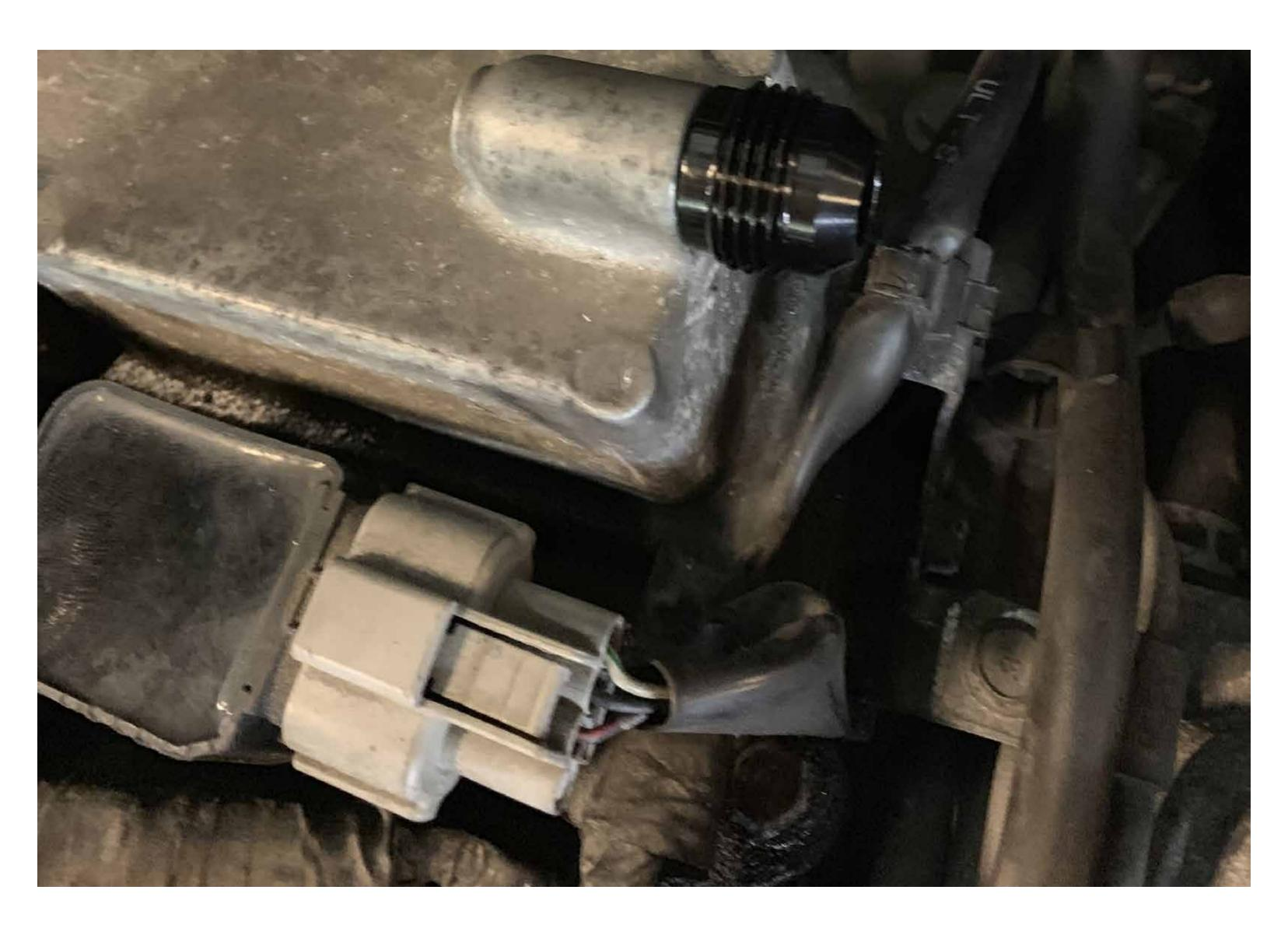
A-B - Press in included -10an fitting into the valve cover by lightly hammering it with a rubber hammer, place a small piece of wood over the fitting to protect it if need be
