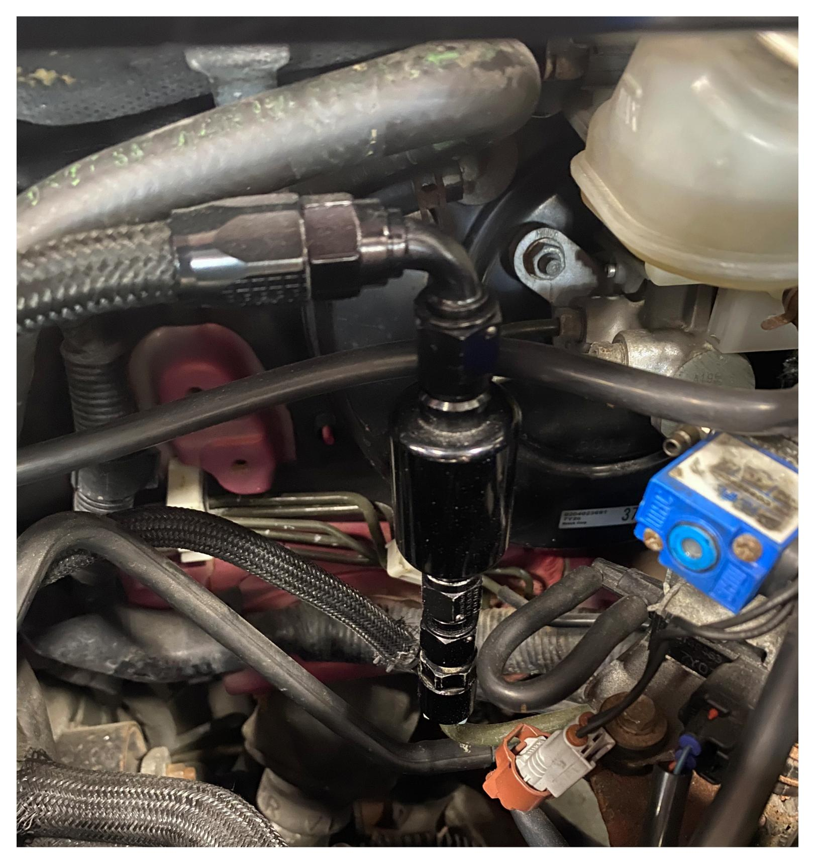
Route the feed line as pictured is the most ideal position. Due to different intakes, and turbo manifolds this can change a little. Press the quick disconnect fitting onto the factory feed line and feel for the same click as the rail side. Reinstall charge piping, leave engine cover off to check for leaks
