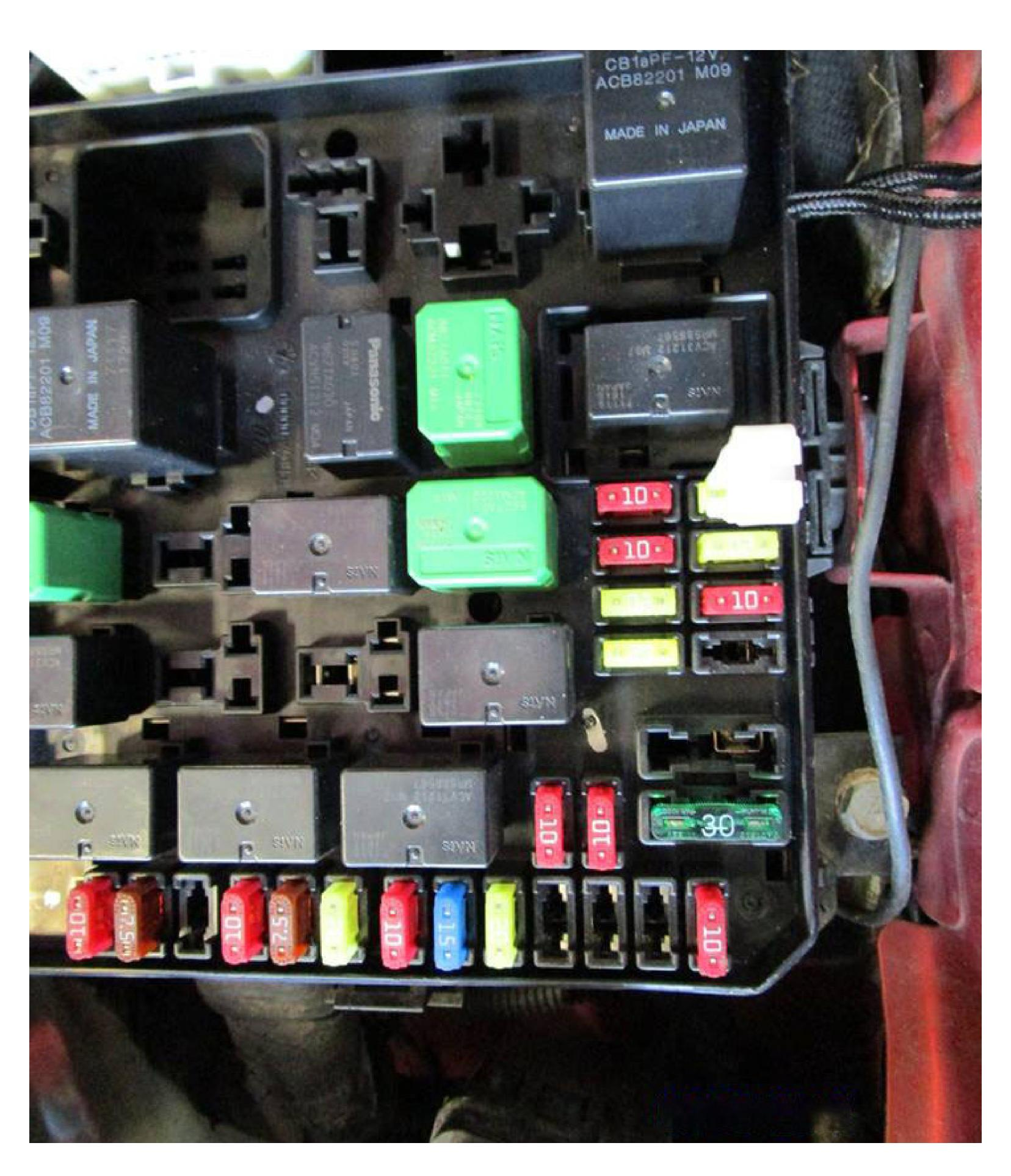
Remove engine cover and charge pipe, set to the side, then remove Fuel pump fuse from underhood fuse block and start, or attempt to start to bleed off any fuel in the lines
