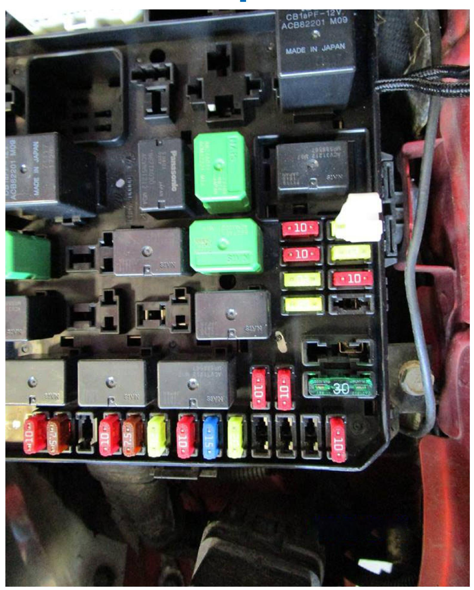
Install fuel pump fuse, power the car on and watch for leaks. If no leaks, install the engine cover and you are good to go!
