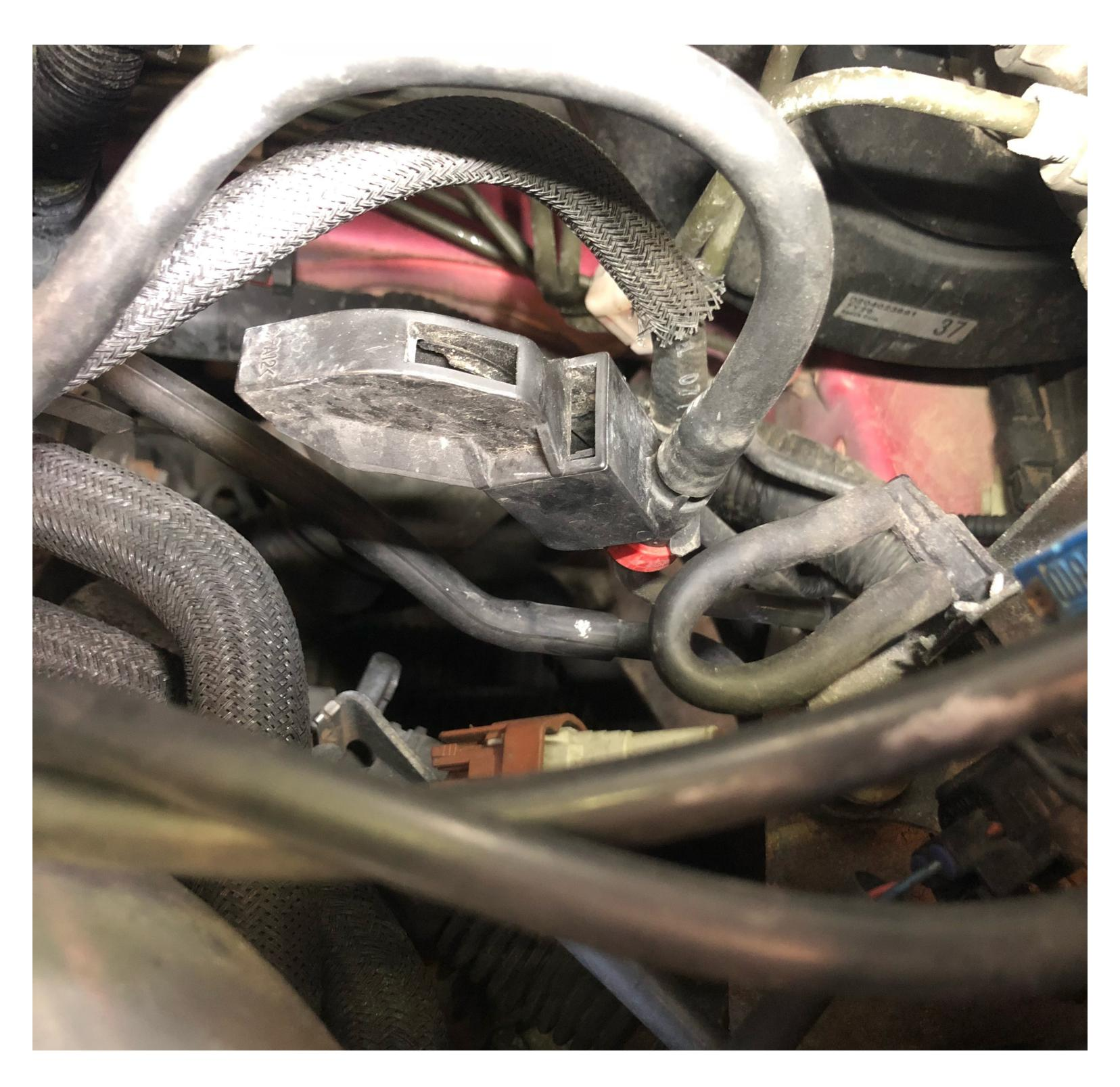
Pull along the lower fuel line to remove the black cover and remove clip that holds the soft line to the factory feed hardline, same as the fuel rail. You may need a pick, but in most cases you can get it by hand. Remove stock line.
