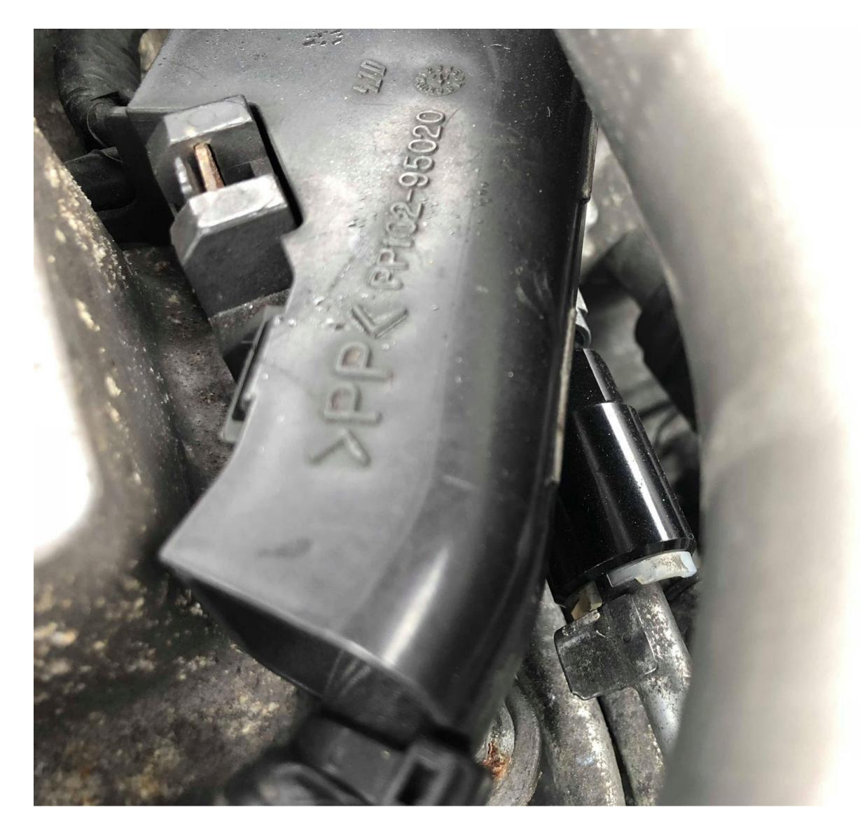
IMPORTANT- You will have to bend the tab on the fuel rail connection to ensure the quick disconnect fitting will properly seat.
