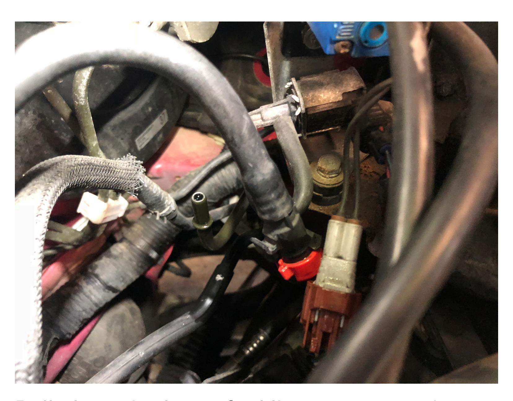
Pull along the lower fuel line to remove the black cover and remove clip that holds the soft line to the factory feed hardline, same as the fuel rail. You may need a pick, but in most cases you can get it by hand. Remove stock line.
