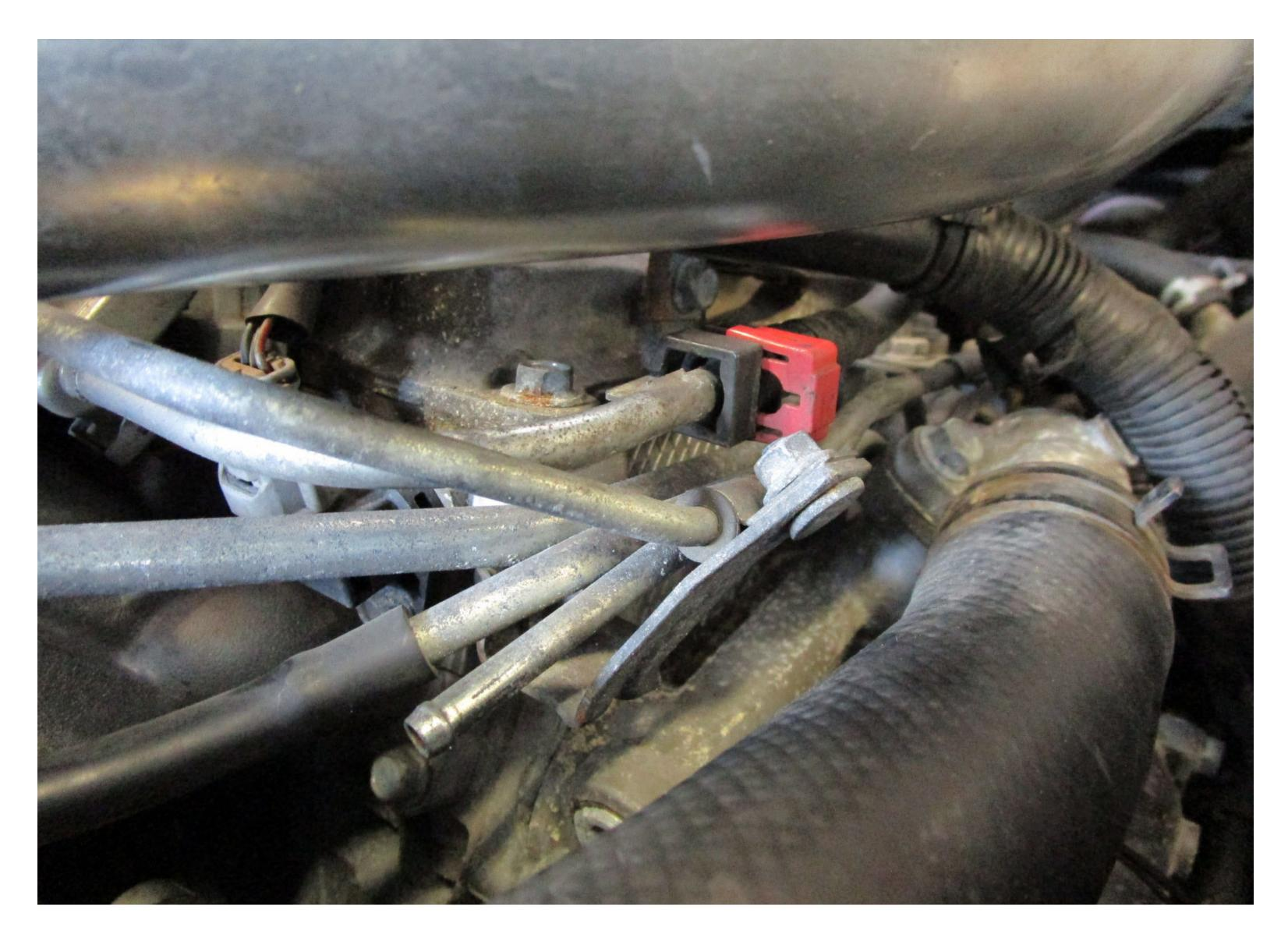
Remove red clip from factory fuel feed line on the fuel rail, you might need a small pick for this but in most cases you can pull it apart with your fingers. Remove line from rail side.
