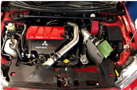
**2. LOOSEN CLAMPS HOLDING THE FRONT COOLER PIPE TO THE INTERCOOLER AND THE REAR UICP**
