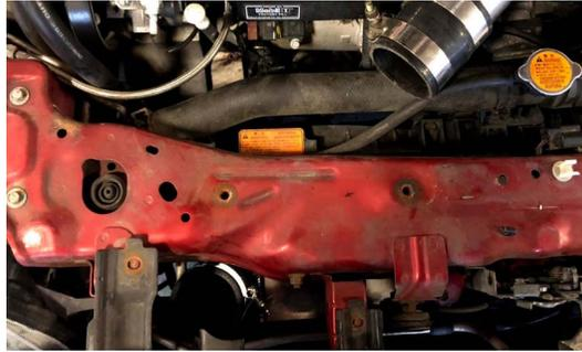
**5. INSTALL MAP FUICP INTO THE NEW COUPLERS, DO NOT TIGHTEN CLAMPS YET**
