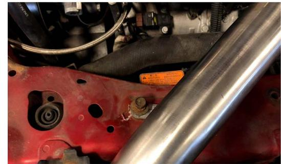
**7. POSITION THE NEW FRONT UPPER PIPE TO YOUR DESIRED FITMENT, THEN START BY TIGHTENING THE MOUNTING TAB BOLT AND THEN TIGHTEN THE T-BOLT CLAMPS, START CAR AND CHECK FOR LEAKS.**
