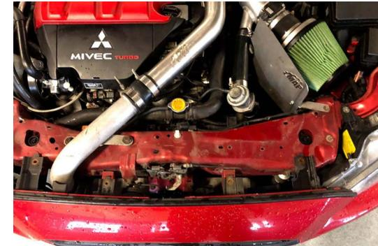
**3. REMOVE 2 BOLTS SECURING FRONT UPPER COOLER PIPE TO THE CORE SUPPORT**
