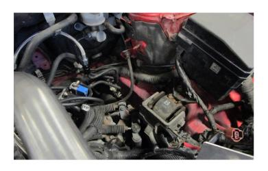
5. REMOVE CLUTCH LINE RETAINING CLIP, TAP WITH A FLATHEAD SCREWDRIVER AND A MALLET TO UNSEIZE THE CLIP, REMOVE WITH A PLIERS OR CHANNEL LOCKS.
