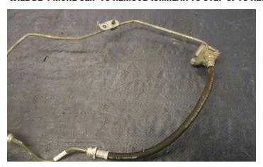
16. INSTALL THE LINES FOR THE FLUID FEED, AND SLAVE CYLINDER ONTO MASTER, LEAVE THE BANJO BOLT LOOSE AS YOU WILL HAVE TO POSITION IT TO CLEAR THE BOOSTER ONCE ASSEMBLED IN THE CAR.
