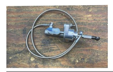
17. INSTALL CMC ASSEMBLY THE SAME AS STOCK, BY TWISTING COUNTER-CLOCKWISE INTO ITS SLOT UNTIL IT CAN NO LONGER ROTATE, THEN TIGHTEN THE LOCKING BOLT.
