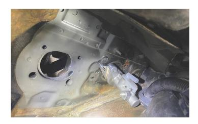
18. WITH THE PEDAL ALL THE WAY OUT, SLIP THE BALL END OF THE ADAPTER CLEVIS OVER THE BALL ON THE PEDAL. IF YOU ARE HAVING TROUBLE INSTALLING THE BALL SOCKET, WE RECOMMEND SLIDING THE RETAINING CLIP OUT OF PLACE, AND STARTING WITH IT AS PICTURED SO THAT ONCE THE INNER RETAINING CLIP SEATS, YOU CAN SLIDE THE EXTERNAL RETAINING CLIP INTO PLACE. YOU SHOULD HEAR A LOUD CLICK ONCE THE INNER CLIP IS SEATED PROPERLY.
