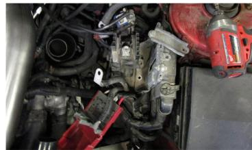
4. UNBOLT ECU BRACKET, AND PULL ASSEMBLY TO THE SIDE. REMOVE BRACKET TRAY, 2 BOLTS AND 1 NUT WILL HOLD IT IN.
