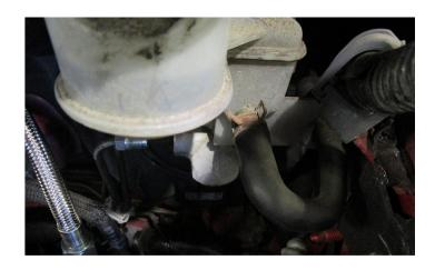
9. REMOVE COTTER PIN AND PIN FROM THE BRAKE PEDAL AND MASTER CYLINDER CLEVIS, AND THE FOUR NUTS AROUND THE PEDAL HOLING IN THE BOOSTER.
