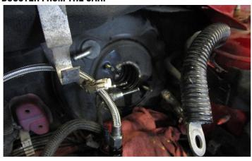
11. USING A FLATHEAD OR PRY TOOL, REMOVE THE MASTER CYLINDER BALL SOCKET FROM THE CLUTCH PEDAL.
