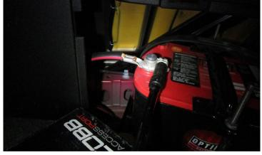
3. REMOVE THE BOOST CONTROL SOLENOID LINES AND ASSEMBLY, SET TO THE SIDE. REMOVE POSITIVE CABLE FROM TERMINAL POST
