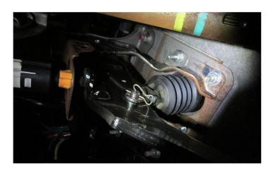
10. REMOVE LEVEL SENSOR CONNECTOR AND THE TWO NUTS HOLDING THE MASTER TO THE BOOSTER, PULL MASTER, AND THEN BOOSTER FROM THE CAR.
