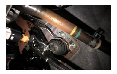
20. INSTALL THE MASTER BACK ONTO THE BOOSTER, ATTACH FEED LINE TO CLUTCH MASTER AND BRAKE LINES TO MASTER, THEN PLUG IN LEVEL SENSOR. AT THIS POINT, YOU CAN TIGHTEN THE BANJO BOLT ON THE CLUTCH MASTER CYLINDER.
