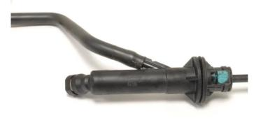
15. REMOVE THE CLUTCH LINE FROM THE SLAVE CYLINDER USING A 10MM LINE WRENCH. WE RECOMMEND REMOVING THE FACTORY CLUTCH FLUID LINE FROM THE VEHICLE AS IT WILL NOT BE REUSED. YOU WILL HAVE TO DESTROY IT TO REMOVE. THERE WILL BE 1 MORE CLIP TO REMOVE (SIMILAR TO STEP 5) TO REMOVE THE SLAVE LINE FROM THE TRANSMISSION.
