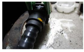
5. UNPLUG WIRING CONNECTOR ON TOP HAT
