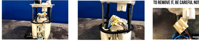
11. REMOVE THE RETAINING RING FROM THE FUEL PUMP ASSEMBLY BY LIFTING THE CLIPS ON THE SIDE AND REMOVE THE PUMP/FILTER ASSEMBLY. Then remove the retaining clips from the filter body.
