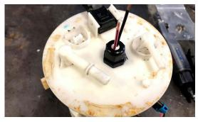
18. RE-INSTALL HOSE FROM FUEL PUMP OUTLET To the top of the fuel pump sending unit 19. REASSEMBLE TOP HAT ONTO BASKET AND INSERT THE C CLIP TO HOLD THE ROD IN PLACE
