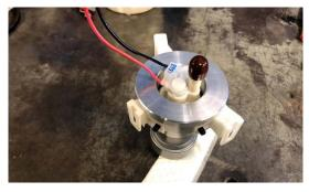
14. PLACE YOUR WIRING BULKHEAD IN THE CENTER OF THE TOP HEAD, WERE IT WON'T BE OBSTRUCTING ANY OTHER LINES. USE PICTURE AS A REFER-ENCE WHERE TO MARK, USE STEP BIT TO DRILL TO APPROXIMATELY ½INCH.
