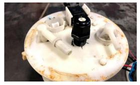
15. SLIDE THE BULKHEAD INTO PLACE, FLIP THE TOP HAT OVER AND MARK WHERE YOU WILL NEED TO GRIND TO ENSURE THE SECURING NUT SITS FLAT, GRIND AWAY UNTIL RETAINING NUT SITS FLUSH ON THE BULKHEAD.
