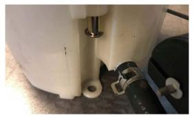
9. DISCONNECT OEM FUEL PUMP FROM THE TOP HAT BY UNPLUGGING The Wiring Harness on the top of the Pump(black and blue wires).
