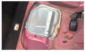
5. UNPLUG WIRING CONNECTOR ON TOP HAT
