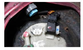
6. REMOVE THE 8MM NUTS HOLDING THE SENDING UNIT TO THE FUEL TANK
