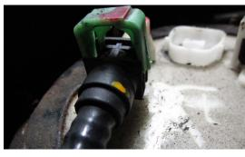
7. PULL SENDING UNIT FROM THE CAR, AND Disconnect fuel line from bottom of Housing (be careful, may be filled with Fuel when pulling out)
