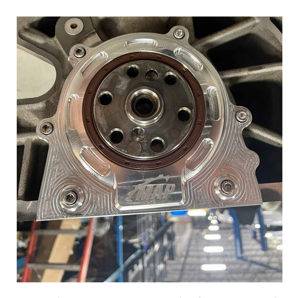
After letting sealant sit for 20 minutes, install MAP EBM-RMH to your engine block, securing with included hardware torqued to 90 inch LBS
