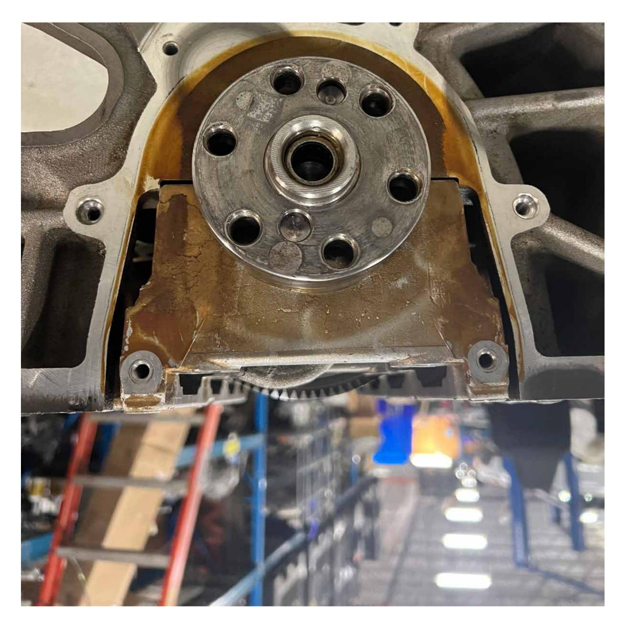
Clean Rear main seal surface. Ensure surface on block is clean, free of oil or leftover sealant.
