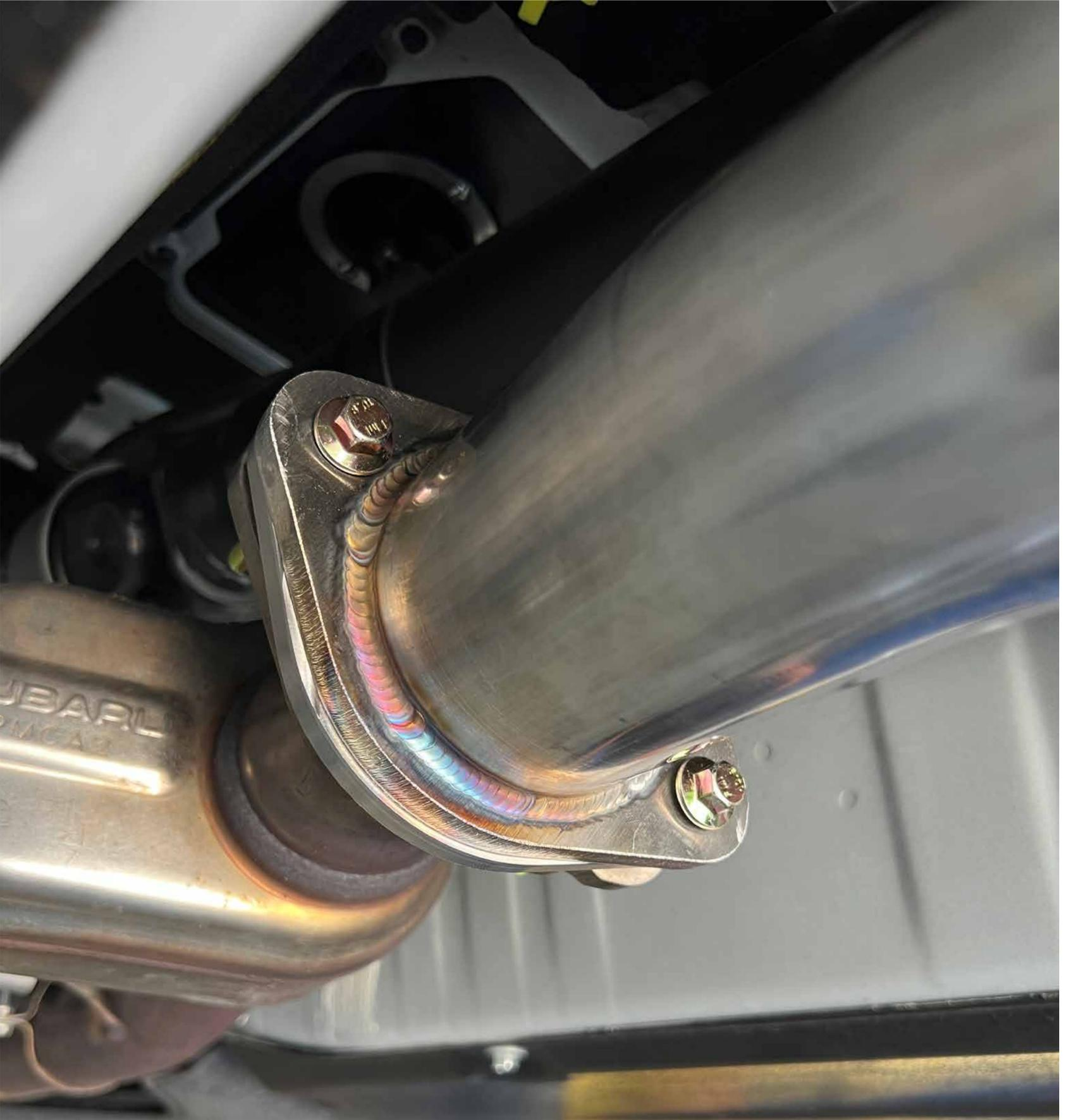
Install MAP Catback front pipe to downpipe. Do not tighten completely. Install Grimmspeed adapter flange if using factory downpipe
