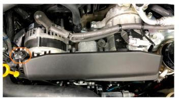
**02.** Install the pulley cover bracket as shown. Re-use the stock 10mm bolt holding the bracket to the alternator and use the included M8 nut and bolt to attach to the black bracket next to the oil filter. Install the bolt from the bottom so that the nut is on top, as shown. Before fully tightening the fasteners, make sure that the bracket is straight and centered. The holes for the fasteners are enlarged to allow small amounts to adjustment.
