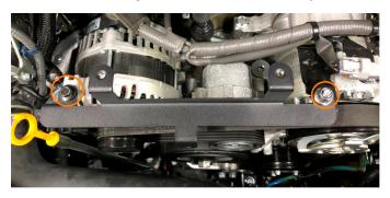
03. Install the pulley cover as shown and fasten with the included 3X M6 Allen bolts and beauty washers using a 4mm Allen key.
