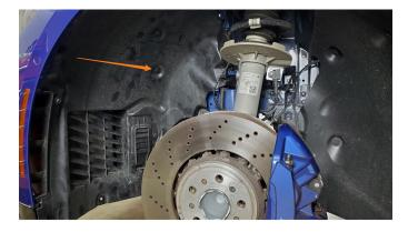
**03.** Using a 10mm socket, remove the bolt securing the air duct to the upper auxiliary radiator bracket. Then, using a 13mm socket, remove the two (2) bolts securing the upper auxiliary radiator bracket and remove the bracket from the auxiliary radiator.
