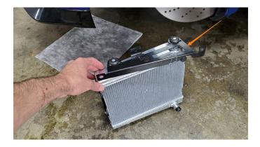
**07.** Remove the dust caps from the inlet & outlet of the Mishimoto auxiliary radiator (if not already done) and install the Mishimoto auxiliary radiator into the vehicle. Using a 10mm socket, secure the air duct to the bracket with the bolt removed in step 3. Then, using a 13mm socket, secure the bracket to the vehicle with the two (2) bolts removed in step 3. Finally, install the upper and lower hoses onto the Mishimoto auxiliary radiator. (Image on next page)
