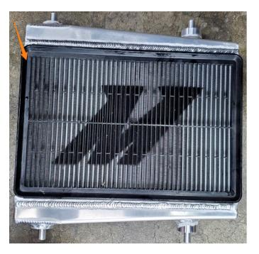
**06.** Install the OEM upper auxiliary radiator bracket onto the Mishimoto auxiliary radiator, as shown below.
