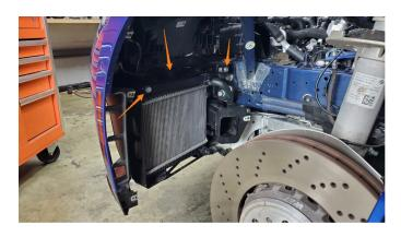
**04.** Drain the coolant into an appropriate container by removing the lower hose from the auxiliary radiator. Then, remove the upper hose from the auxiliary radiator and remove the auxiliary radiator from the vehicle. Properly dispose of the used coolant.
