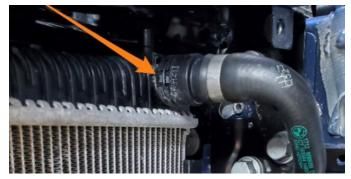
**05.** If Mishimoto rock guards (sold separately) are not being used, transfer the OEM rock guard from the OEM auxiliary radiator to the Mishimoto auxiliary radiator.
