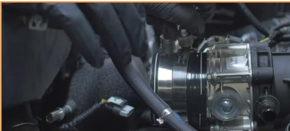
33. Tighten the clamps on your cold-side pipe.
