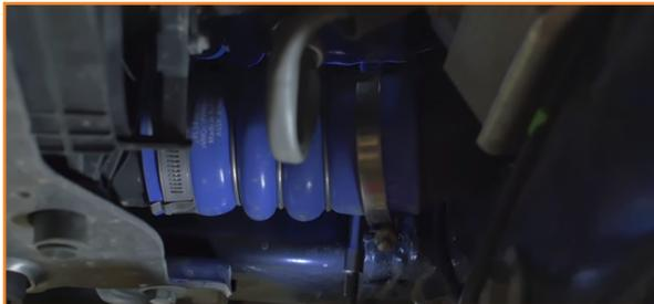
10. Separate the cold-side pipe connector from the intercooler. Pull the clip out of the connector to release it from the intercooler. (1x spring clip)
