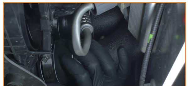
27. Attach the smallest transition coupler to the turbo port. (1x 44-67mm worm gear clamp)
