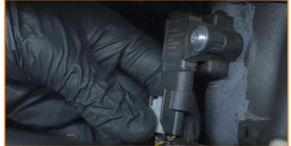
13. Release the clips that secure the sensor's wiring. (2x tree clips)
