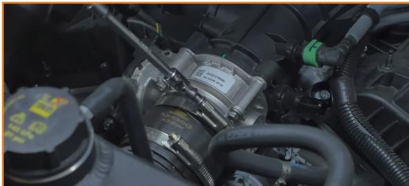
12. Disconnect the air temperature sensor on the cold-side pipe. Depress the tab at the center to separate the connection.
