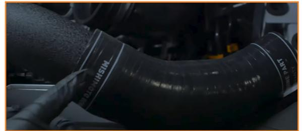
26. Feed the pipe past the front of the engine down to the intercooler. The end without the coupler goes down first and connects to the lower coupler on the intercooler.
