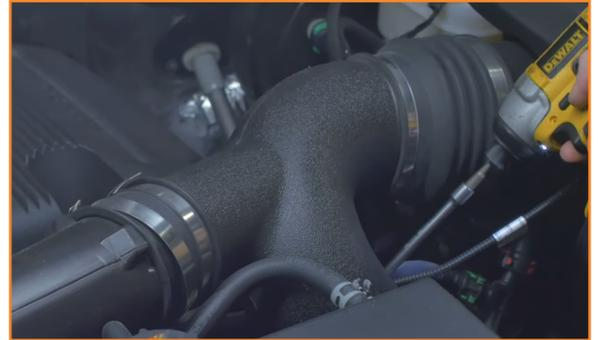
3. Disconnect the air temperature sensor on the intake.
