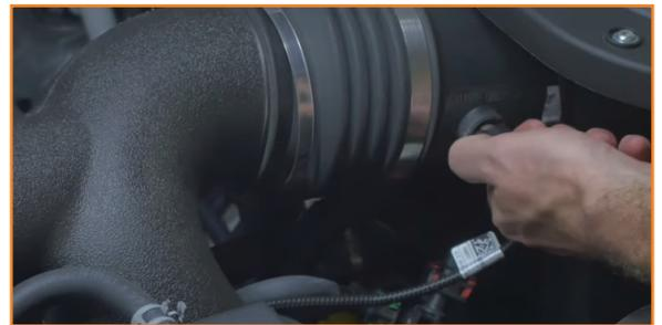
4. Remove the loosened portion of the air intake.
