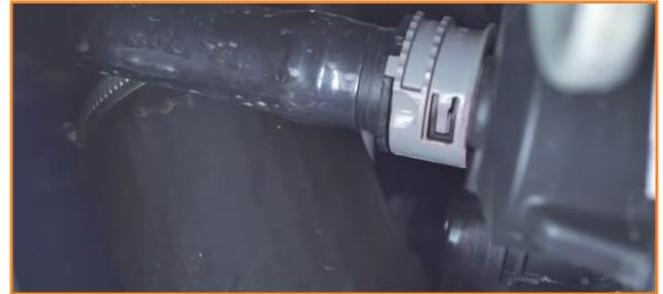
16. Loosen the clamp that secures the cold-side pipe connector to the rest of the piping. Slide the connector out of the piping to remove it. (1x worm gear clamp)
