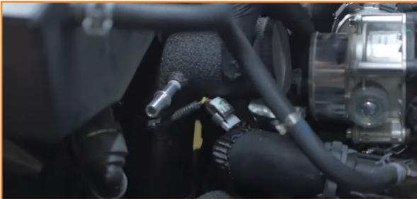
32. Connect the cold-side pipe to the throttle body using the small coupler.
