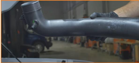
18. Lift the two upper portions of the hot-side piping out of the engine bay. This pipe will also need to be adjusted as you pull it from the engine bay.
