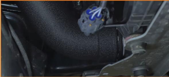
31. Add the 90° section of the cold-side piping to the end of the section already installed to the intercooler. (1x 70-92 worm gear clamp)
