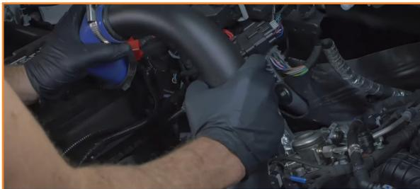
19. Install the Mishimoto couplers to the hot-side end tank on the intercooler. Leave the clamps loose for now. You will tighten them later.
