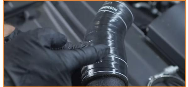
24. Mate the open end of the pipe to the coupler end of the previously installed hot-side pipe. This pipe should then line up with the turbo.
