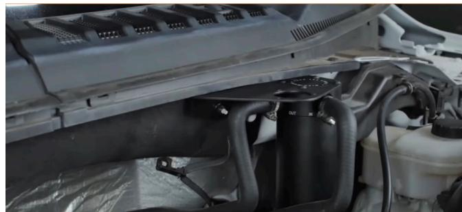
**15.** Attach the 3oz catch can to the bracket using the hardware in your kit. (3x 2.5mm Allen bolts)
