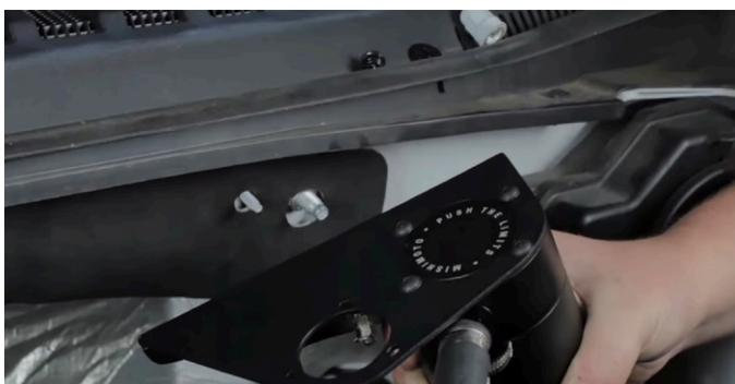
**14.** Secure the bracket to the firewall. Place the ground strap back over the stud, and then set the bracket over the two studs. (1x 15mm acorn nut, 1x 10mm nut and washer)
