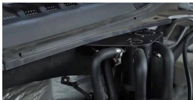
**17.** Remove the oil fill cap to reinstall the engine cover. Then replace the oil fill cap.
