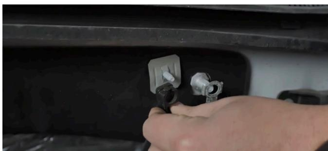
**11.** Connect MM4652-04 to the OUT port on the 12oz catch can. (1x worm gear clamp)
