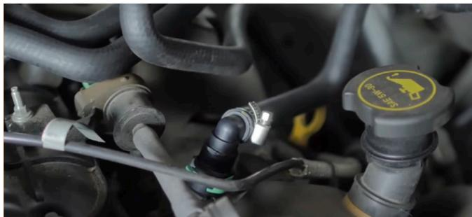
**10.** Remove the nut that secures the ground strap to the firewall. Then slide the plastic prop and metal plate off the nearby stud. (1x 15mm acorn nut)
