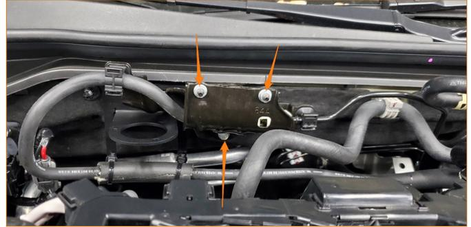
8. Using a 2.5mm Allen key, attach the Mishimoto catch can to the catch can bracket with the three (3) supplied M4 bolts.
