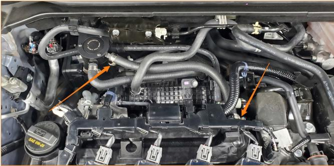
**11.** Use the two (2) supplied hose clips to separate the hoses and keep them from rubbing on one another, as shown in the photo below.
