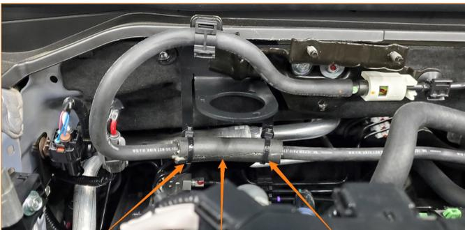
7. Using a 10mm socket, reinstall the front part of the stock bracket with the two (2) nuts and one (1) bolt that were removed in Step 2.
