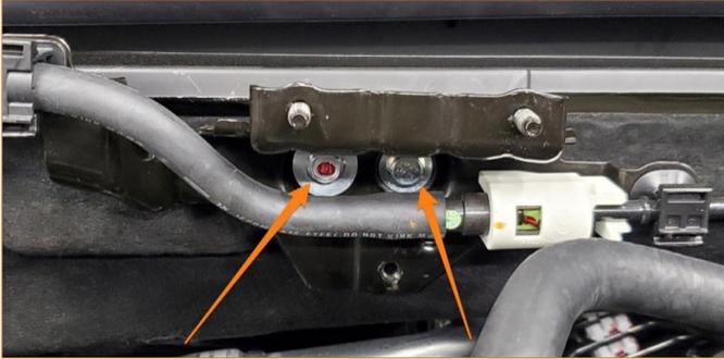
5. Install the catch can bracket behind the rear part of the fuel hose bracket and secure both brackets with the bolts that were removed in the previous step.
