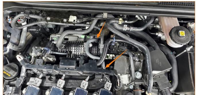
3. Using a 10mm socket, remove the two (2) nuts and one (1) bolt securing the front part of the two-piece fuel hose bracket on the firewall. Remove the front part of the bracket to gain access to the bolts securing the rear part of the bracket to the vehicle.
