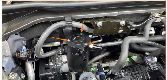
9. Install the shorter end of the supplied bent hose to the port on the catch can labeled "OUT" and secure it with one (1) of the supplied worm gear clamps. Install the other end of this hose to the port on the intake manifold and secure it with one (1) of the supplied worm gear clamps. The worm gear clamps can be tightened using a 7mm socket or a flathead screwdriver.
