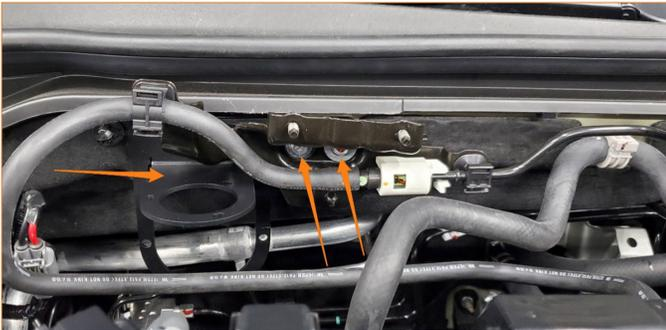
6. Place the split hose over the stock fuel hose that runs in front of the catch can bracket. Use the two (2) supplied tree clip zip ties to secure the fuel hose to the catch can bracket, as shown in the photo below.
