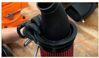
11. Assemble the passenger-side air intake by inserting the tube assembly into the heat shield. Push the rubber grommet lip all the way around to fully seat it in the heat shield.
