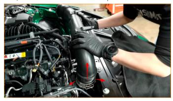
08. Install the Mishimoto aluminum turbo snout on the passenger-side turbo. Fasten with stock hardware.
