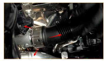
**04.** Loosen the two E8 Torx bolts, then remove the aluminum turbo snout from the passenger-side turbo.
