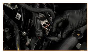
22. Tighten the remaining worm gear clamp.
