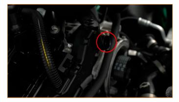
20. Install the driver-side intake assembly. Line up the intake tube with the silicone coupler, then push down on the heat shield to engage the bottom rubber grommets.
