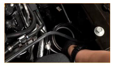
19. Temporarily disconnect the electrical harness shown to gain more clearance when installing the driver-side intake.
