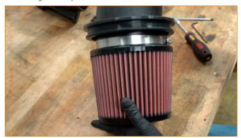
**14.** Assemble the driver side air intake by inserting the tube assembly into the heat shield. Push the rubber grommet lip all the way around to get fully engage it into the heat shield.
