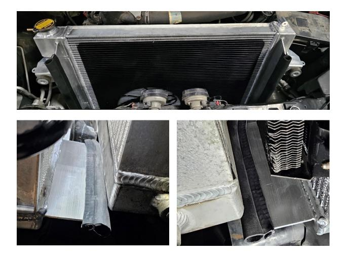
22. Install the supplied trim seals onto the radiator. The 13" trim seal go on the upper stand off aluminuim plates and the 7.5" go on the lower stand off aluminuim plates.
