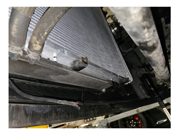
13. Remove the power steering cooler from the radiator.
