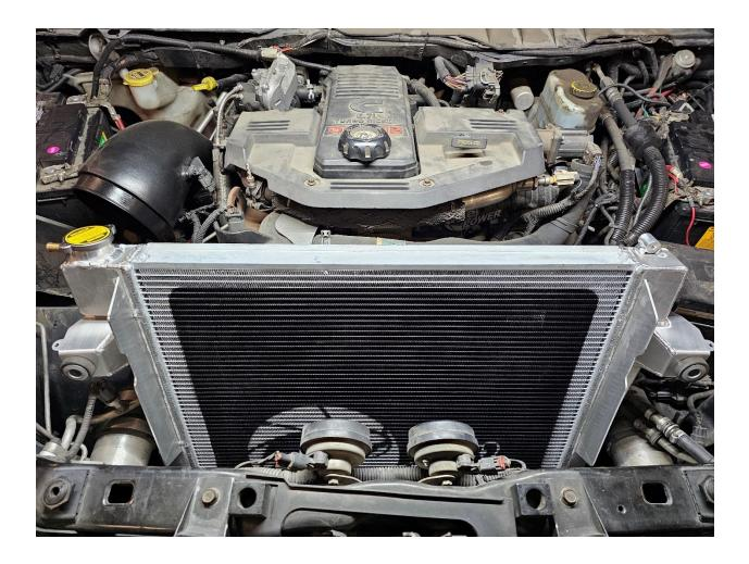
21. Install the aFe Radiator into the truck but do not tighten.
