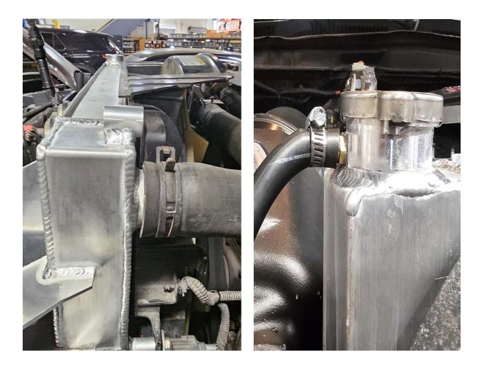
31. Install the upper radiator hose onto the radiator using the OE clamp.
