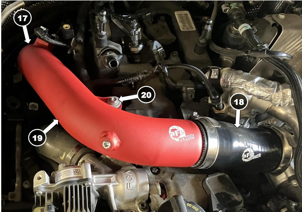
**Note: Be sure to thoroughly clean all oil residue off of the connections before installing any of the aFe POWER couplings onto the vehicle.**
