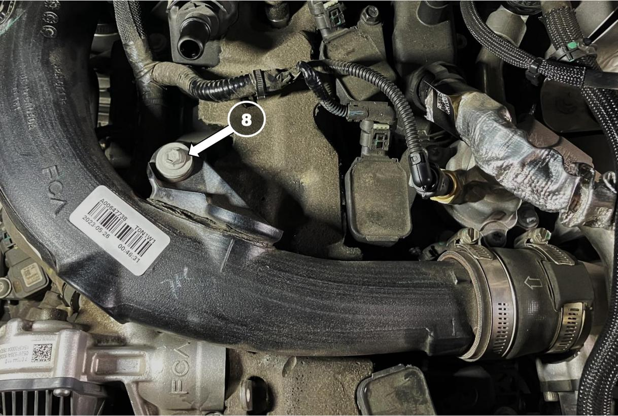
9. Remove the screw securing the charge pipe to the vehicle ⑧
