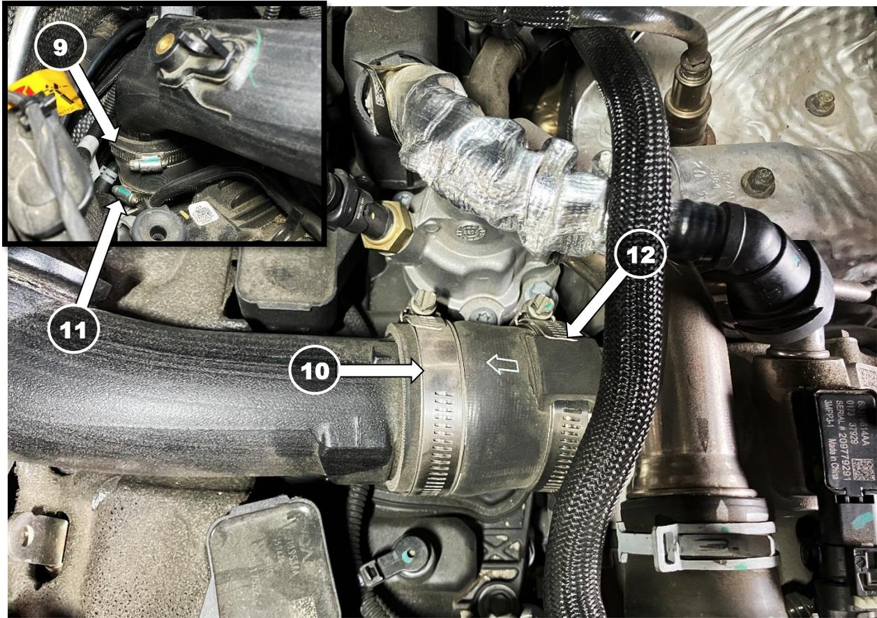
10. Loosen the clamp securing the throttle body coupling onto the charge pipe (9).
