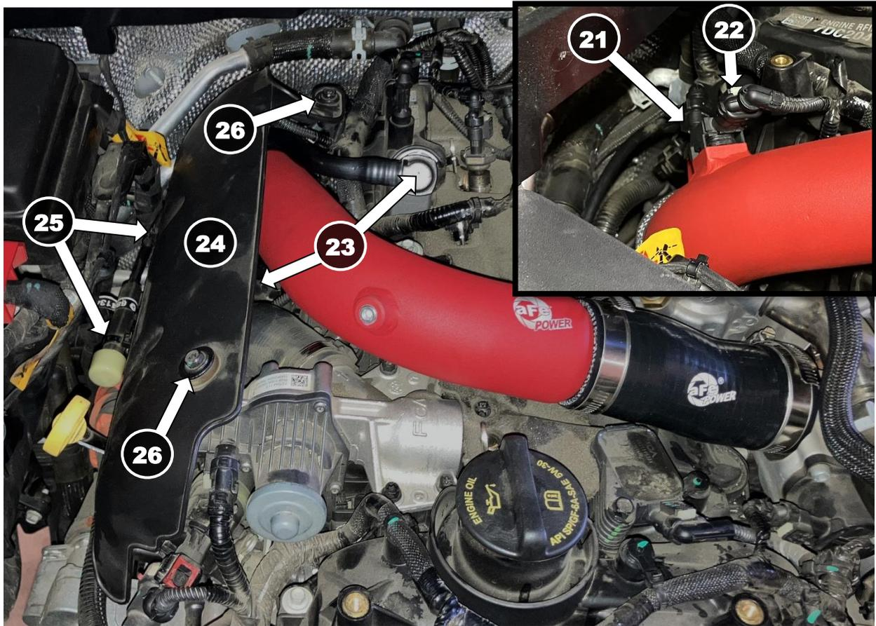
25. Reconnect the temperature sensor connector, then engage the security tab (21).
