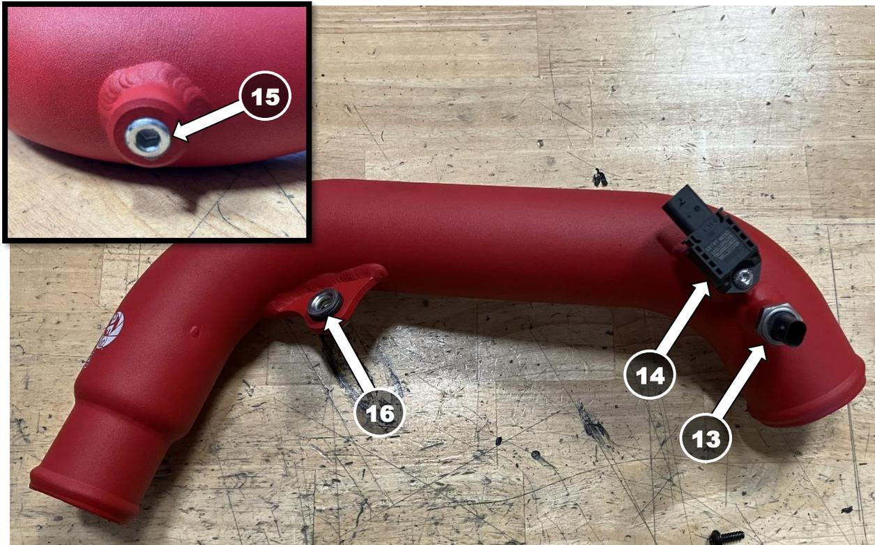
**Note: Be sure to lubricate the O-ring with grease to prevent it from tearing during installation.**
