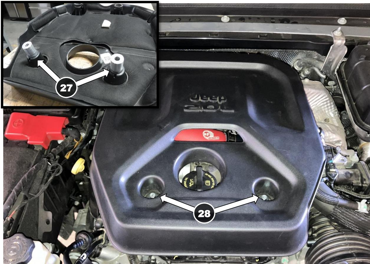
31. Remove the two factory metal insert from the bottom side of the engine cover grommets.
