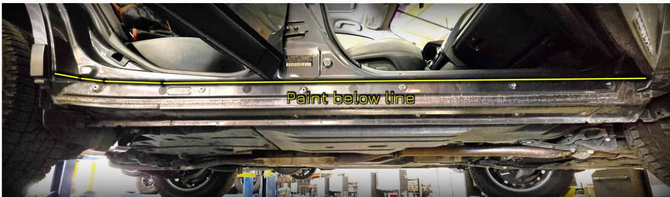
8. Next, install the rivet nuts. The (6) M6 rivet nuts will go on the top vertical portion of the rocker and the (6) M8 rivet nuts will install on the bottom section of the panel.
