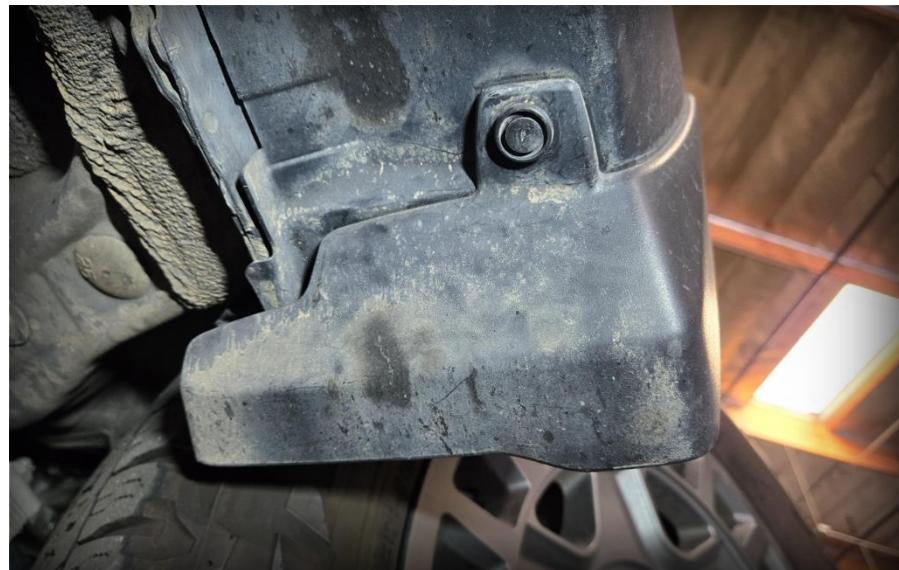
3. Remove the (6) pop clips at the bottom of the rocker panel.
