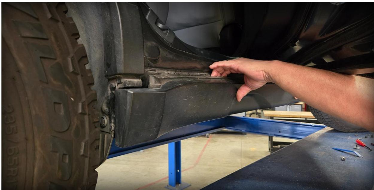
5. Toward the front of the rocker cladding, at the bottom of the front fender, there (2) tricky push clips that need to be squeezed to release. Peel open the wheel well plastic to access the backside of these clips. You will need to pinch the two tangs on the clip to release. If you try to just pull on the plastic rocker cladding, you will end up separating the cladding from the clips, still leaving you with the chore of removing the clips from the fender.
