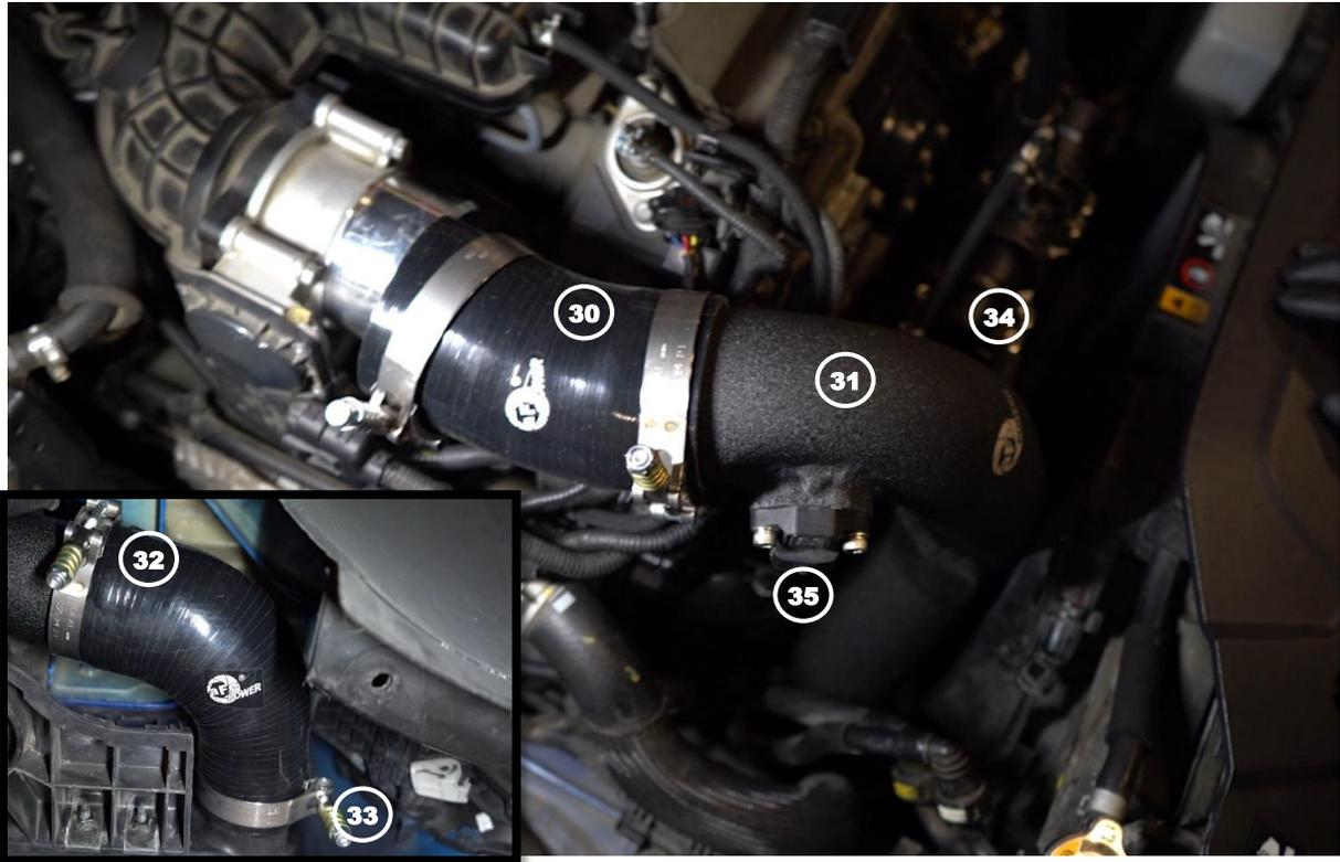
39. Install the supplied aFe silicone reducer elbow (3.15" x 3") 20° to the cold side charge pipe (30) with one 3.25" - 3.5" spring-loaded T-bolt clamp and one 3.5" - 3.75" spring-loaded T-bolt clamp for the throttle body. Do not tighten clamps yet.
