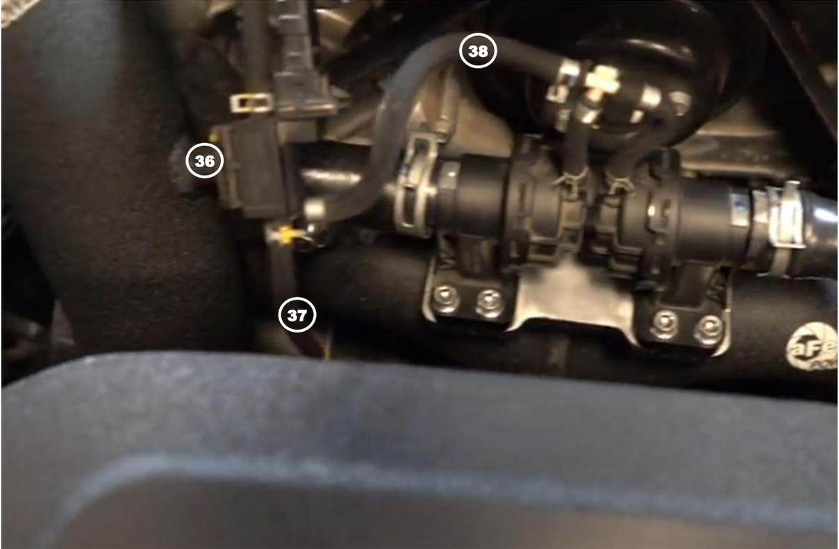
46. Mount the vacuum distribution block onto the cold side aFe charge pipe (36) using the supplied socket head cap screw: M6x1.0x12 and M6 washer.
