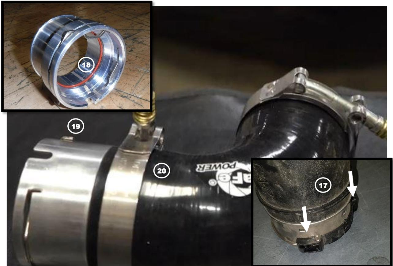
**Note: The retaining clip will need to be removed from the factory charge pipe for reuse with the aFe charge pipe**
