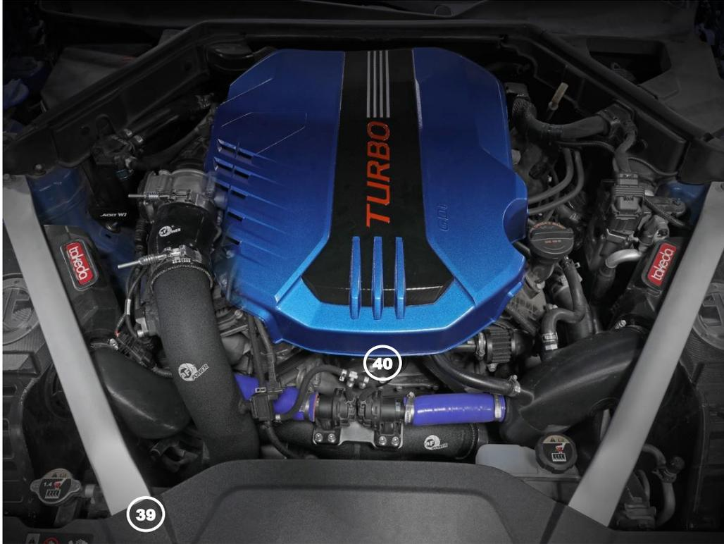
52. Reinstall the strut braces into the vehicle (39)
