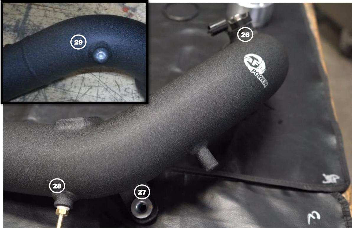
35. Transfer the factory Manifold Pressure Sensor from the factory charge pipe to the supplied aFe cold side charge pipe (26) and secure it using the two of the supplied M6 screws and washers
