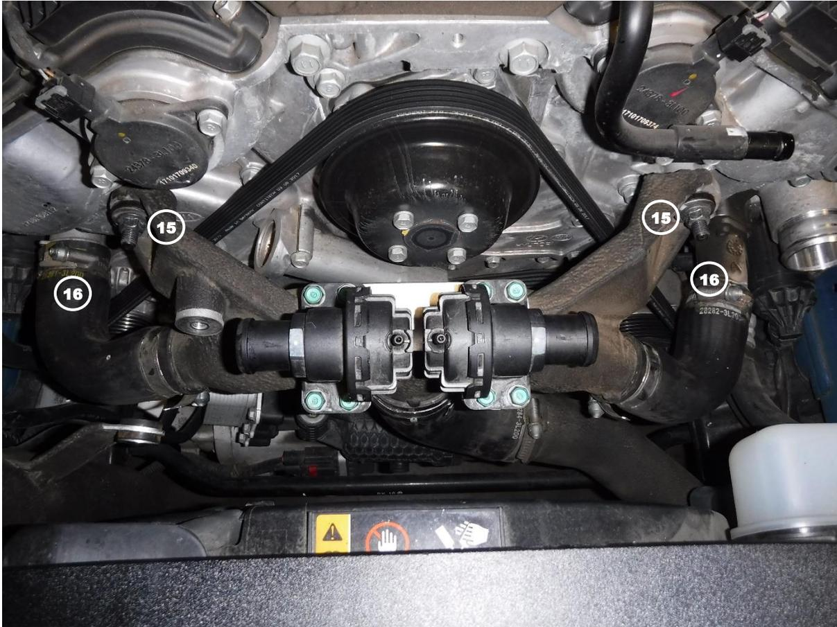
20. Remove the two nuts securing the hot side charge pipe to the engine (15)
