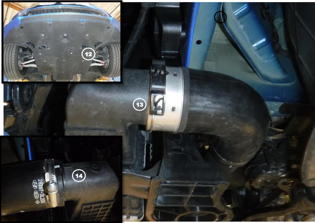
16. From underneath the vehicle, remove all screws and retaining clips securing the belly pan (12) and remove it from the vehicle.
