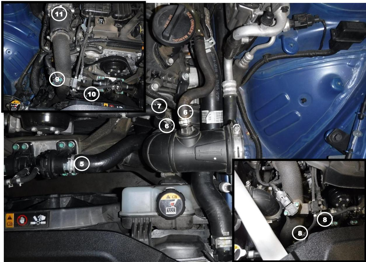
8. Disconnect the bypass hoses from the diverter valves (5).
