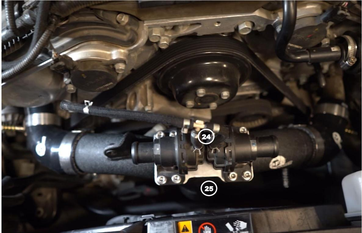
33. Install the diverter valves onto the aFe charge pipe using the supplied socket head cap screws: M6x1.0x20 and M6 washers (24).
