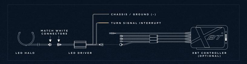
NOTE: The chassis / ground wire must be grounded to bare metal for the LED halo to function properly.
