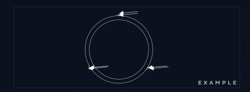
Using installation wire, beading wire, or fishing line, feed the wire from behind the housing/bezel, up and through the MicroMount, then back down through the housing/bezel. Then secure the halo by twisting the wire behind the housing or bezel.
